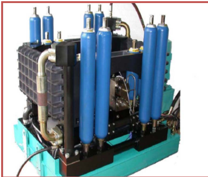
ACTIDYN Earthquake Simulator MODEL QS 67-2 Payload: 1m x 0.5m x 0.6m, 400kg mass
