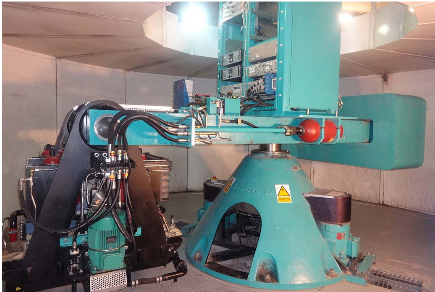
150 g-tonne beam centrifuge (Actidyn C67-2)
