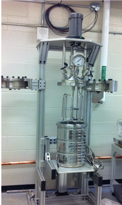
16 L large batch reactor for liquefaction of biomass into bio-crude oils (5kg per batch)
