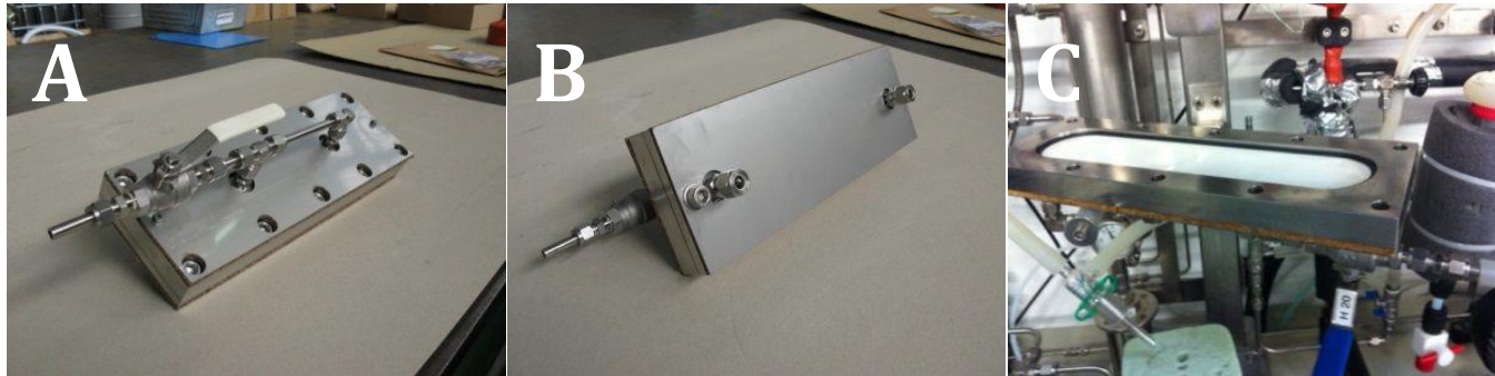
Figure 3.2: Pervap 4060 membrane and test cell: (A) Assembled test cell showing permeate (vacuum) connection, (B) assembled test cell showing feed and retentate connections, (C) test cell permeate part showing sinter plate, membrane and O-ring installed.
