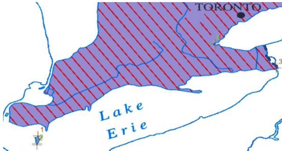
Figure 18: Four control points for georeferencing procedure are shown as the red and green crosshairs.
