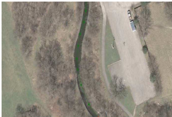
Figure 2.5 Digitizing of river center line using Aerial Photo
