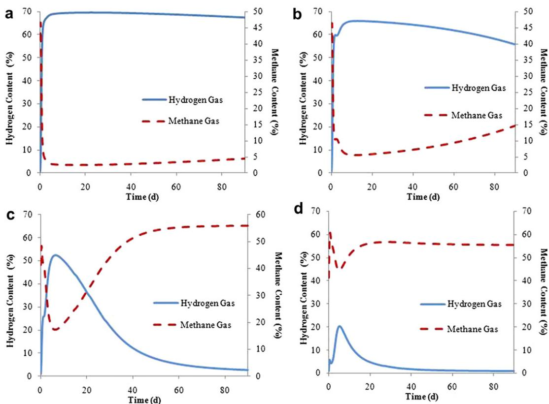
Fig. 6 – Diurnal variations in biogas content at OLR-1 = 6.5 gCOD/L-d and methanogens-ON for a) SRT = 3 days, b) SRT = 5 days, c) SRT = 10 days, d) SRT = 20 days.
