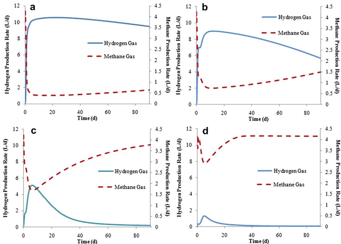
**Fig. 5 – Diurnal variations in biogas production rate at OLR-1 = 6.5 gCOD/L-d and methanogens-ON for a) SRT = 3 days, b) SRT = 5 days, c) SRT = 10 days, d) SRT = 20 days.**
