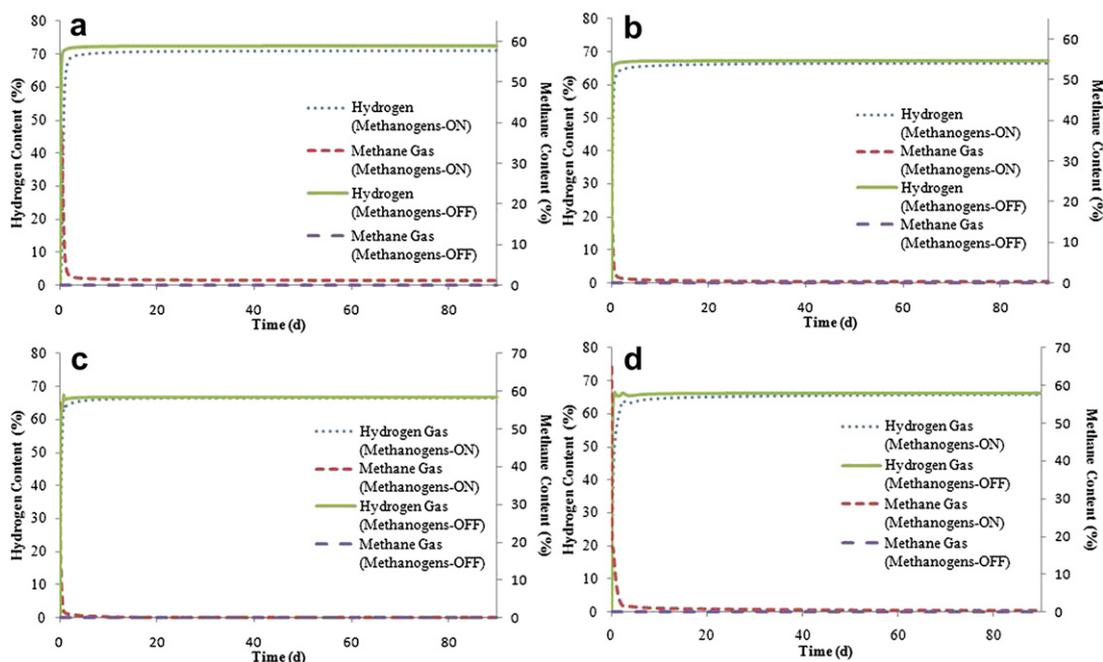
**Fig. 4 – Dynamic simulations for biogas content at: a) OLR-1 = 6.5 gCOD/L-d, b) OLR-2 = 25.7 gCOD/L-d, c) OLR-3 = 51.4 gCOD/L-d, d) OLR-4 = 103 gCOD/L-d.**
