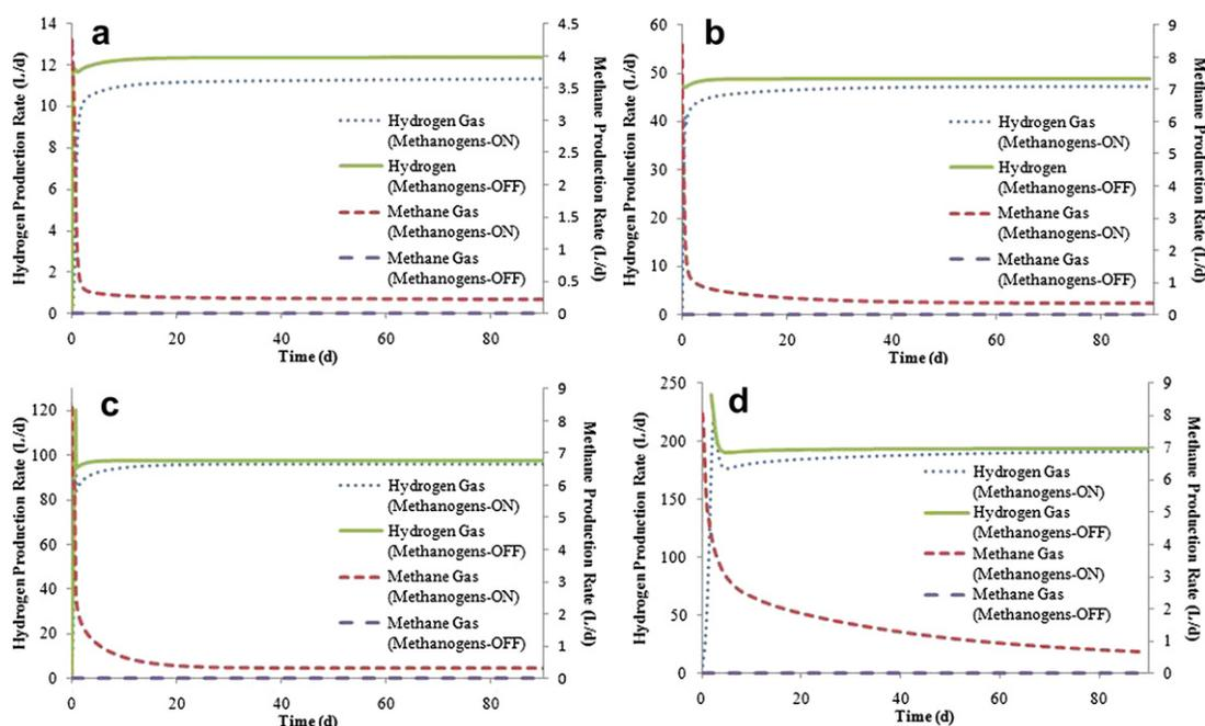
**Fig. 3 – Dynamic simulations for hydrogen and methane production rates at: a) OLR-1 = 6.5 gCOD/L-d, b) OLR-2 = 25.7 gCOD/L-d, c) OLR-3 = 51.4 gCOD/L-d, d) OLR-4 = 103 gCOD/L-d.**
