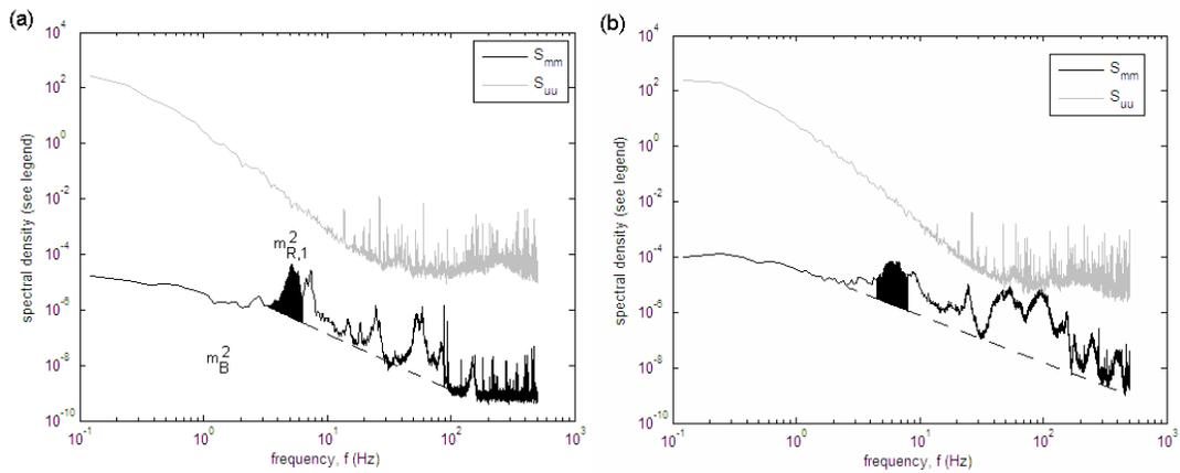
Figure 2. Boundary layer fluctuating wind speed and tower response spectra with a conductor-height mean wind speed of (a) 3.5 m/s and (b) 6.7 m/s.
