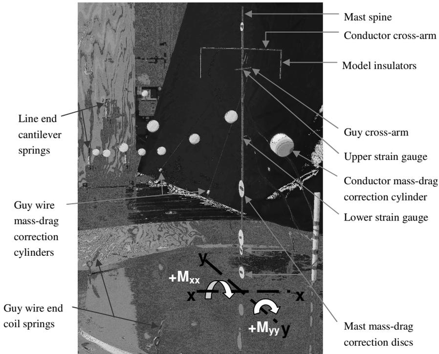
Figure 1. Assembled aeroelastic model.
