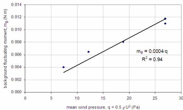
Figure 3. The variation of the background component of tower response with boundary layer mean wind pressure.
