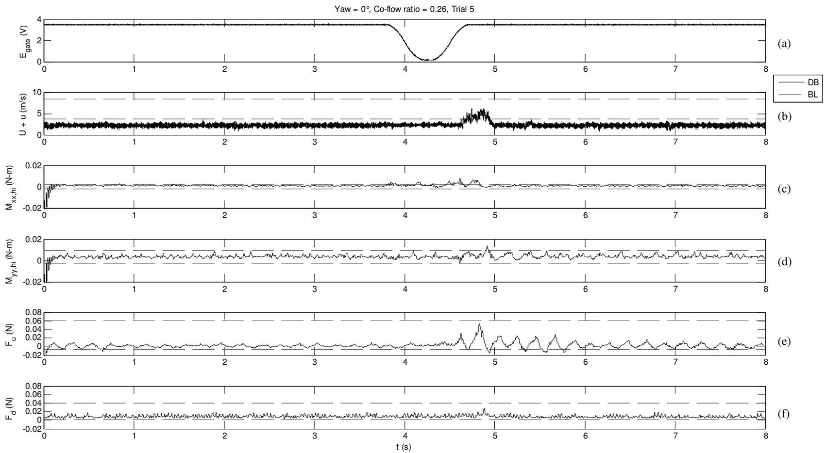
Figure 4. Synchronized histories of measured (a) slot gate position, (b) streamwise velocity, (c) spine bending moment about the x-x axis, (d) spine bending moment about the y-y axis, (e) upstream conductor axial force and (f) downstream conductor axial force.
