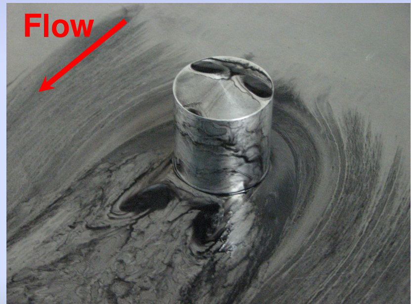
Oil film surface flow visualization of square and circular section cylinders with aspect ratio of AR = 1
