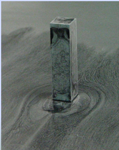
Oil film surface flow visualization of square and circular section cylinders with AR = 4
