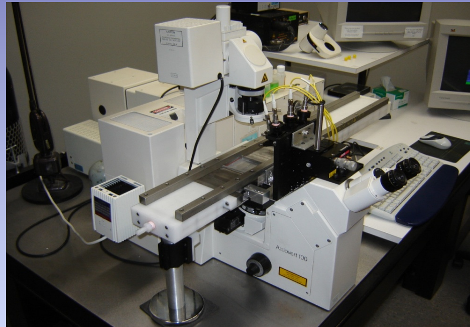
Hemo-dynamic rig mounted on the Laser Scanning Confocal Microscope (LSCM) stage
