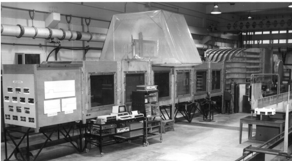
Example of a short test section, open return wind tunnel (fetch of approx 6m)
