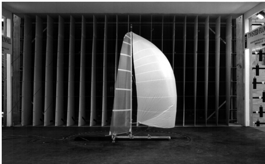
Figure 8. Downwind sail testing in the Twisted Flow Wind Tunnel.
