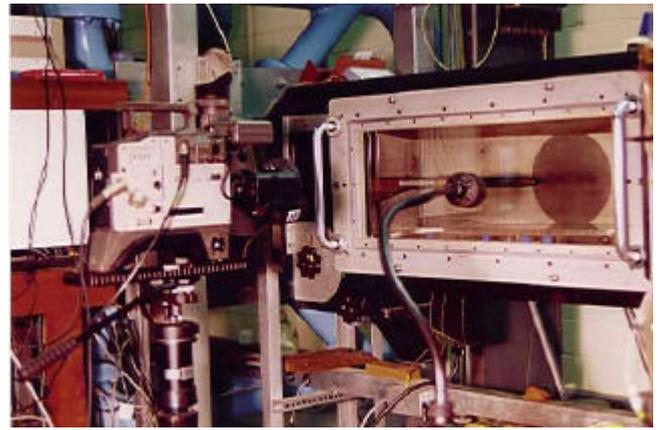
Figure 5: Typical arrangement of tungsten halogen spotlamp and colour video camera
