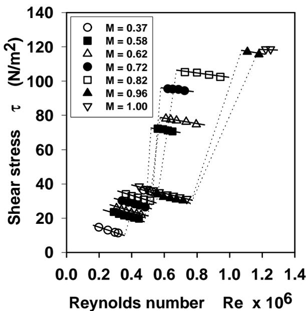
Figure 11: Variation of shear stress with  $Re$  for the different Mach numbers
