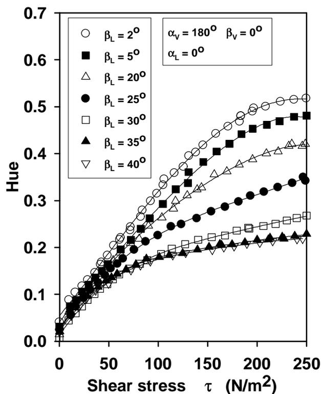
Figure 8: Variation of hue-shear calibration with changes in vertical illumination angle
