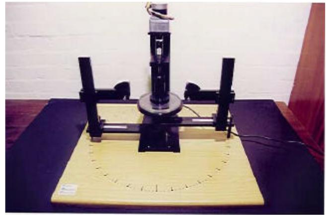
Figure 2: General overview of the complete rotational shear rig and probe holders
