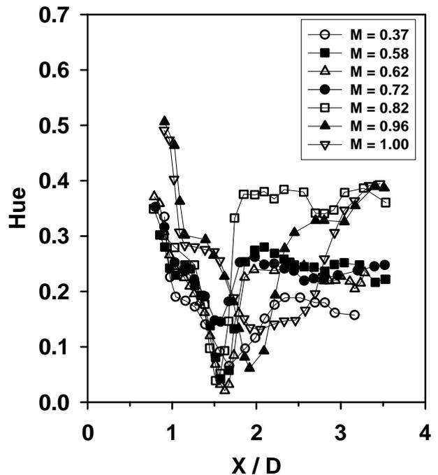
Figure 10: Variation of hue with distance along model axis at different Mach numbers
