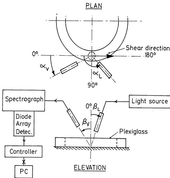
Figure 1: Layout of spectrophotometric apparatus and lighting/viewing angle conventions
