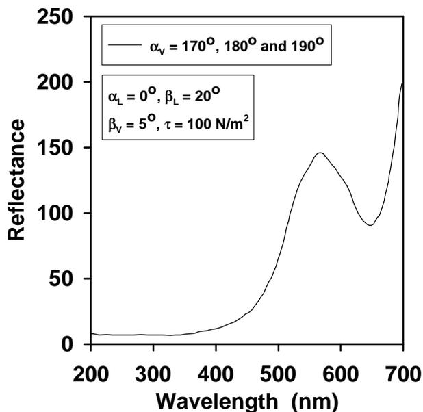
Figure 7: Variation of spectrum with change in horizontal viewing angle for constant shear
