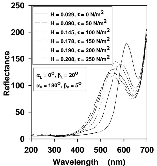
Figure 6: Variation of spectrum with increase in shear for fixed optical conditions
