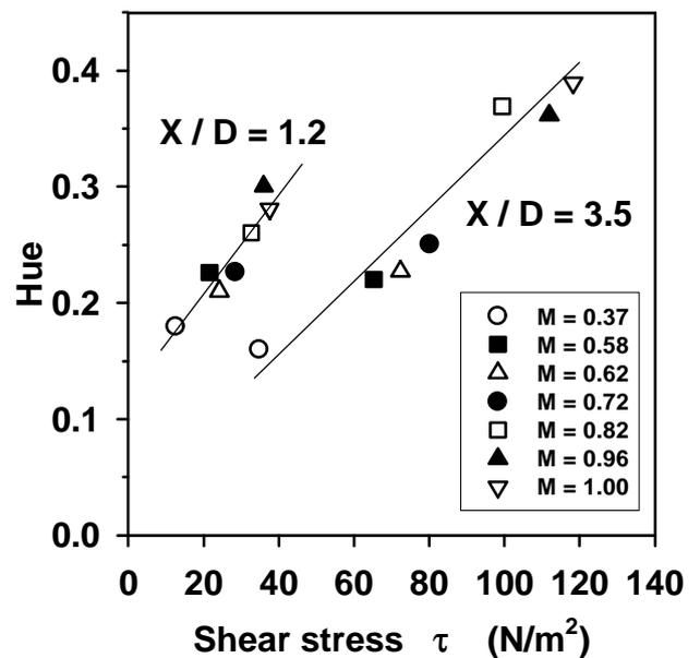
Figure 12: Variation of hue with shear stress for two locations on the model
