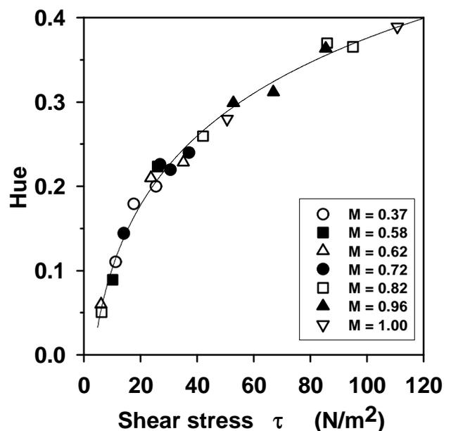
Figure 13: Variation of hue with shear stress taking into account illumination angle
