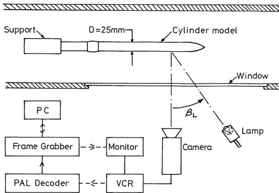
Figure 3: Diagrammatic layout of apparatus for wind tunnel tests
