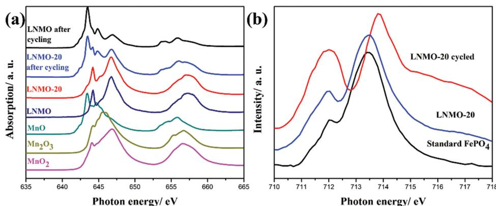
Figure 5. a) XANES Mn  $L_{3,2}$ -edges of LNMO-20, LNMO-20 cycled, LNMO-0, LNMO-0 cycled, and standard MnO,  $Mn_2O_3$ ,  $MnO_2$ ; b) Fe  $L_3$ -edges of standard  $FePO_4$ , LNMO-20 and LNMO-20 after 100 battery cycles collected in TEY mode.
