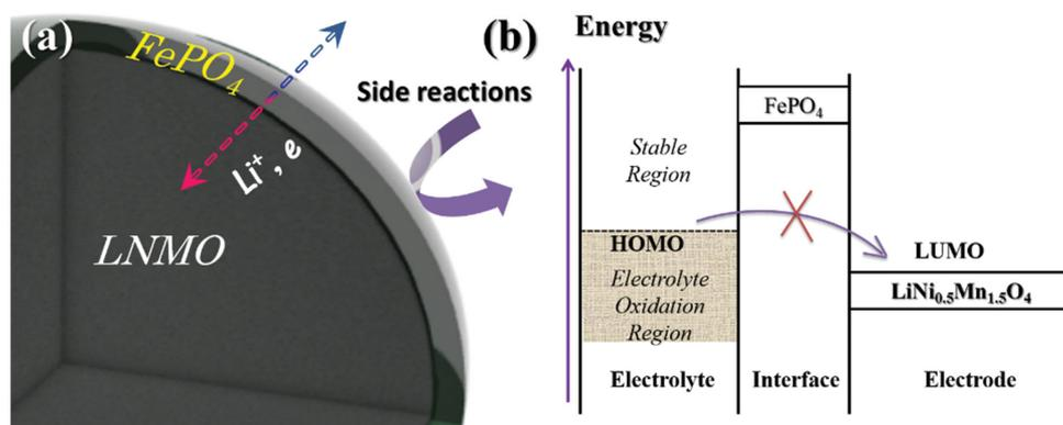
**Figure 6.** Schematic illustrations of a) LNMO-*n* upon cycling; b) illustration of the electrolyte highest occupied molecular orbital (HOMO) and work functions of FePO<sub>4</sub> and LiNi<sub>0.5</sub>Mn<sub>1.5</sub>O<sub>4</sub>.
