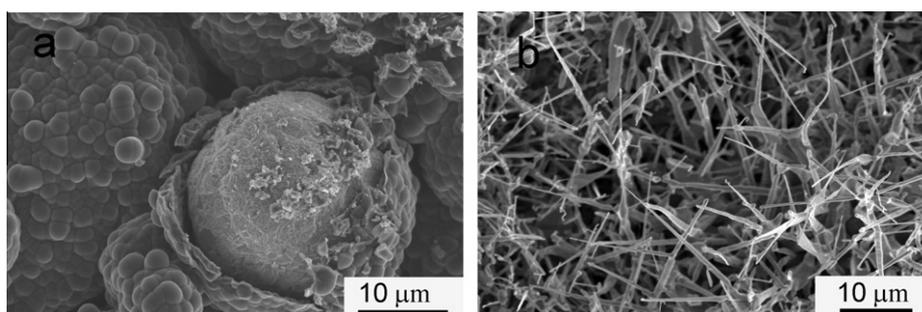
Fig. 5. SEM images of sample synthesized with (a) pure acetone and (b) pure water.
