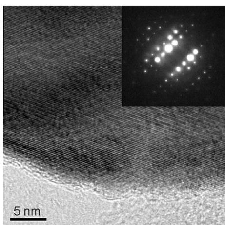
Fig. 3. HRTEM image and related selected area diffraction pattern of the synthesized structure.
