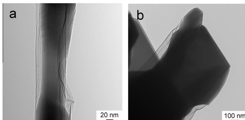
Fig. 2. TEM images of  $\text{TiO}_2$ @C nanostructures: (a) nanorod and (b) nanowall.
