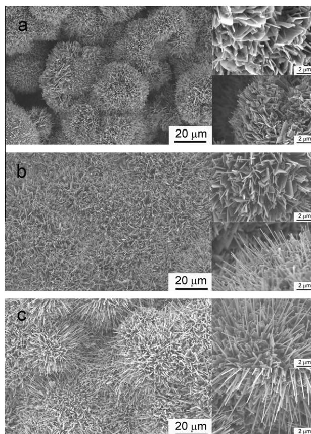
**Fig. 1.** SEM images of  $\text{TiO}_2$ @C nanostructure grown at (a)  $850\text{ }^\circ\text{C}$ , (b)  $900\text{ }^\circ\text{C}$  and (c)  $950\text{ }^\circ\text{C}$  for 2 h respectively on titanium powder without catalyst. The picture at the up-right corner is a high magnification top-view image and the picture at the down-right corner is a high magnification side-view image.
