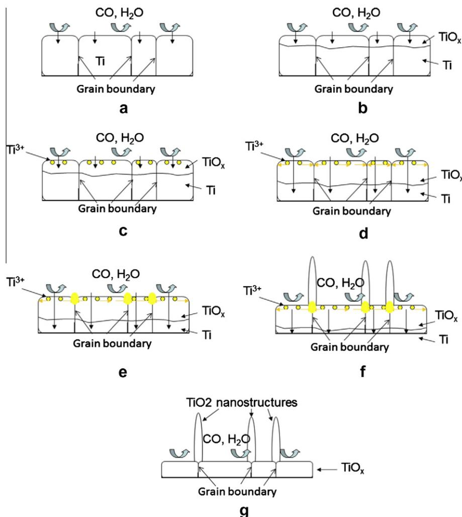
Fig. 6. Schematic illustration of the growth steps of carbon covered  $\text{TiO}_2$  nanostructures. Black arrows are showing the diffusion direction of oxygen atom and yellow arrows are showing the diffusion direction of Ti cations. (For interpretation of the references to color in this figure legend, the reader is referred to the web version of this article.)
