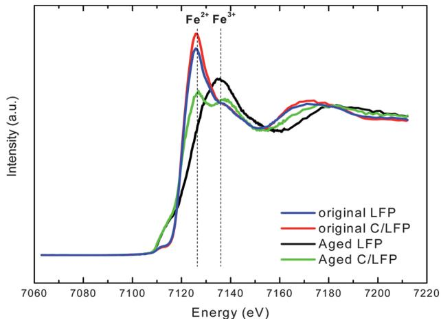
Fig. 8 Fe K-edge XANES spectra of  $\text{LiFePO}_4$  samples.
