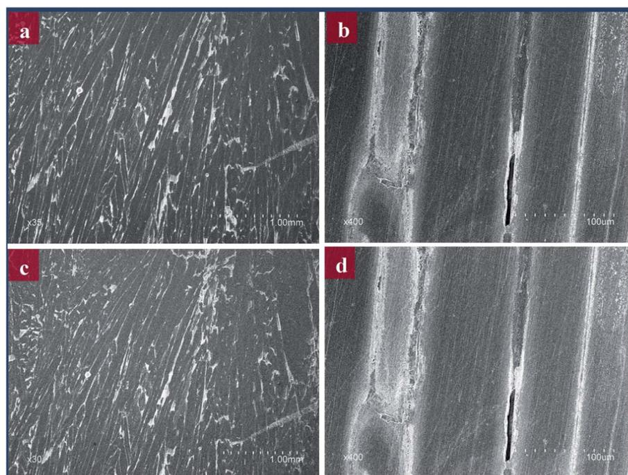
**Fig. 6** SEM images of  $\text{C/LiFePO}_4$  before (a and b) and after 32 h (c and d) the aging process.
