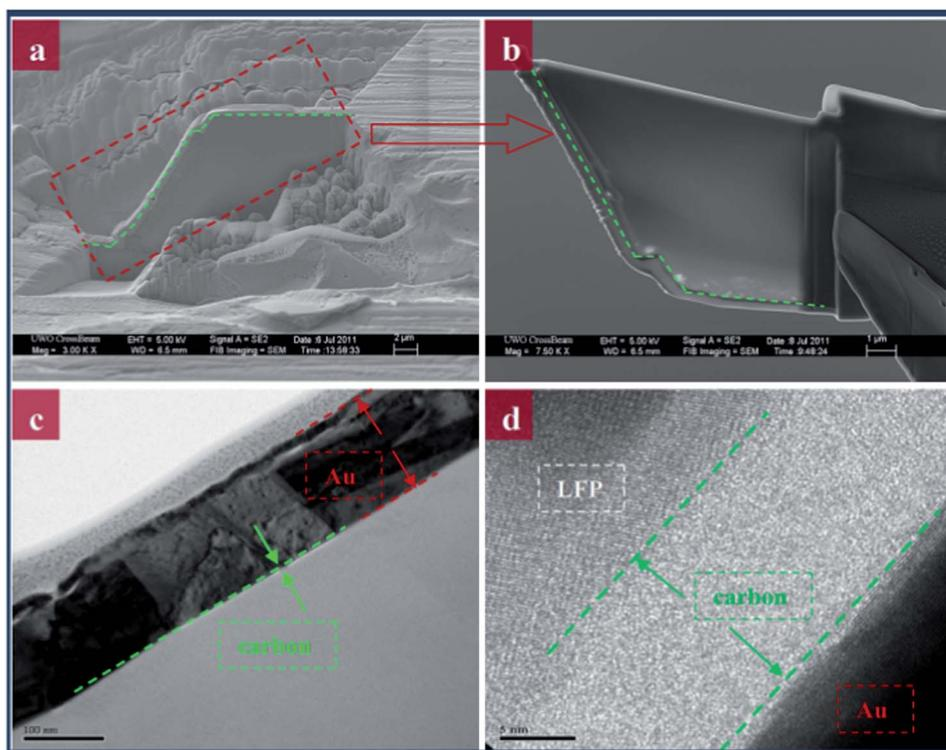
**Fig. 5** SEM images of the FIB sample (a and b), TEM (c), and HRTEM (d) images at the carbon layer zone on the FIB sample.
