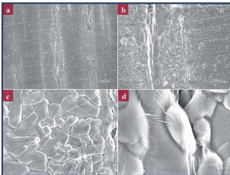
Fig. 4 SEM images of carbon coated  $\text{LiFePO}_4$  with different magnifications.
