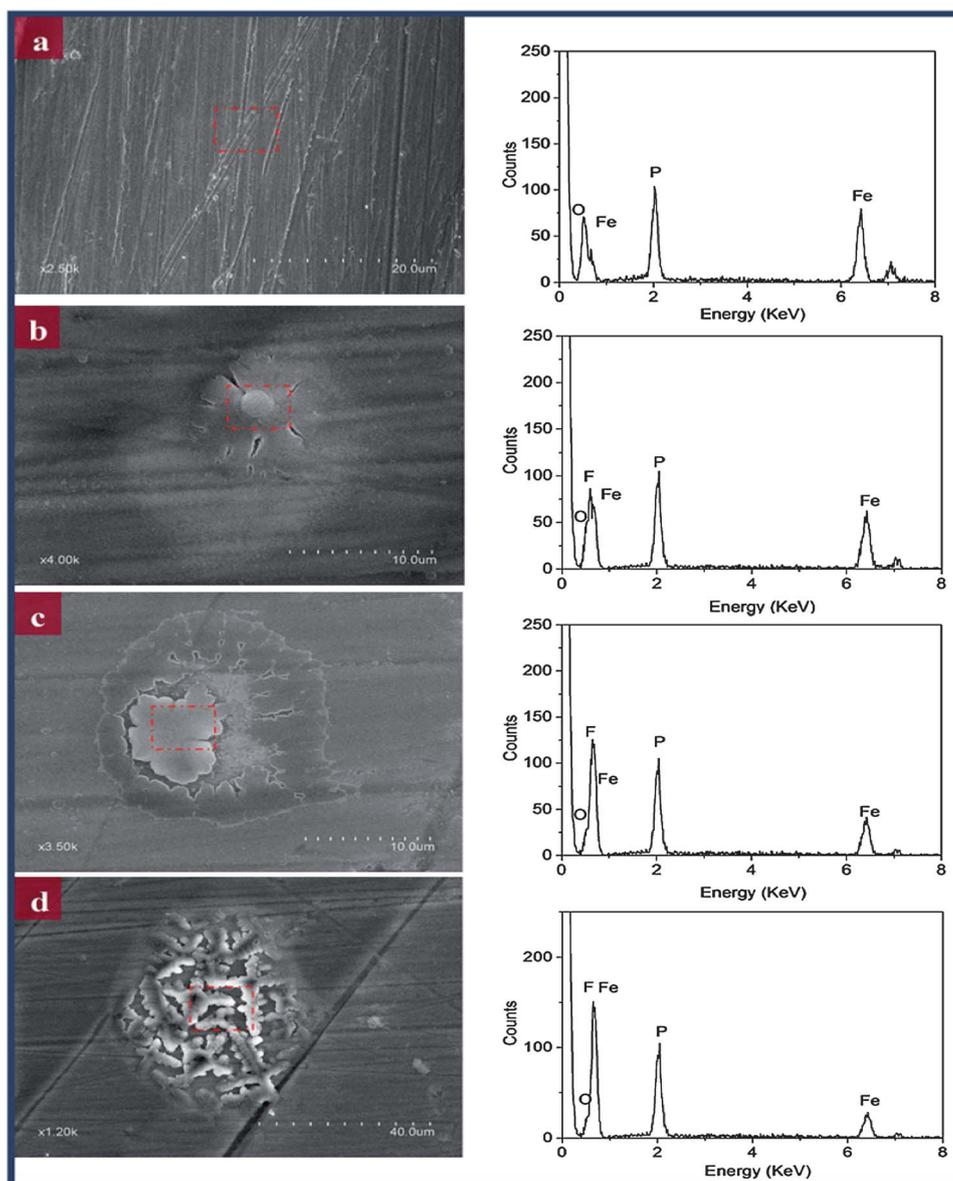
Fig. 2 Iron element dissolves on the  $\text{LiFePO}_4$  surface during the surface aging process at 0 h (a), 8 h (b), 24 h (c) and 32 h (d).
