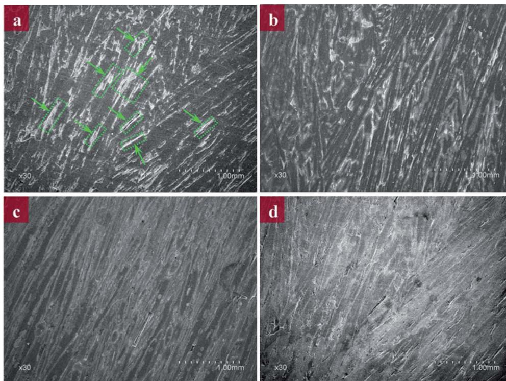
**Fig. 1** SEM images of the  $\text{LiFePO}_4$  surface during the surface aging process at 0 h (a), 8 h (b), 24 h (c) and 32 h (d).
