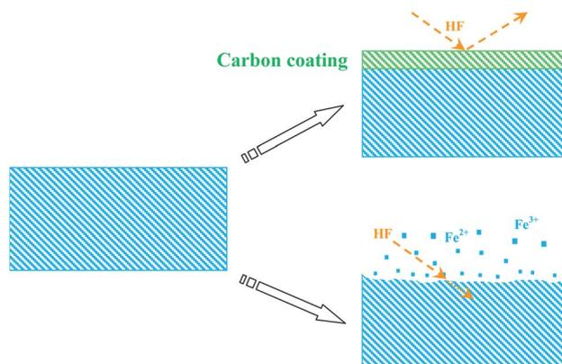
Fig. 9 Schematic diagram of surface corrosion at pristine  $\text{LiFePO}_4$  and carbon coated  $\text{LiFePO}_4$ .
