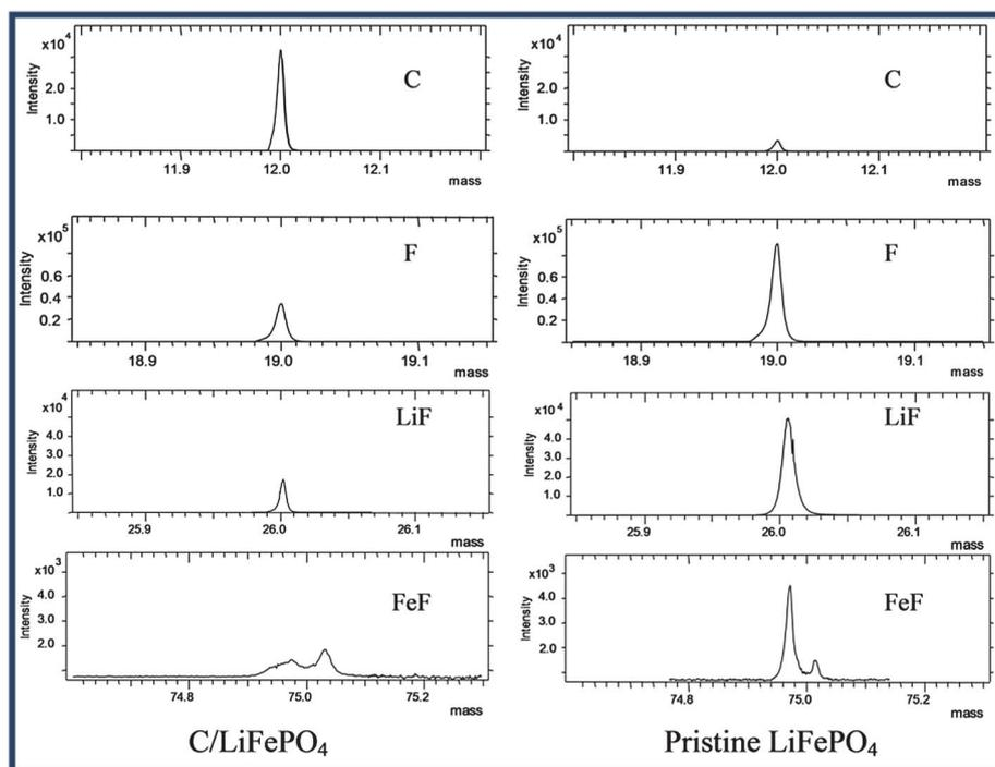
Fig. 7 ToF-SIMS mass spectra of the two aged samples.
