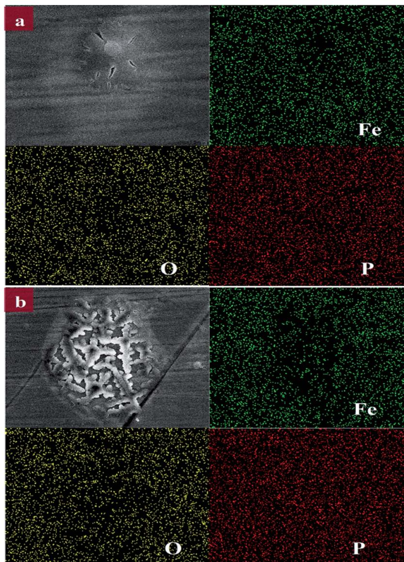
Fig. 3 Element mapping of iron element dissolving during the aging process at 8 h (a) and 32 h (b).
