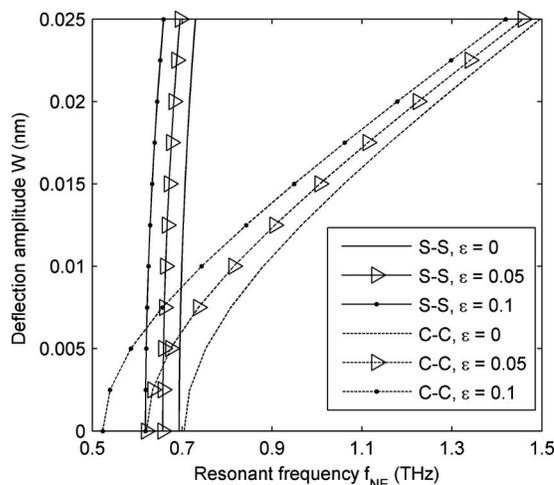
FIG. 5. Effect of the axial load on the resonant frequencies of an embedded CNT ( $d=0.7$  nm and  $L=20$ ).
