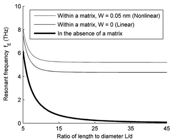
FIG. 8. Variation in the resonant frequencies of an embedded CNT with the  $L/d$  ( $d=0.7$  nm).
