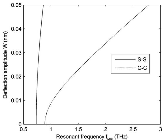
FIG. 1. Vibrational mode of an embedded CNT with different end conditions ( $d=0.7$  nm and  $L=10d$ ).
