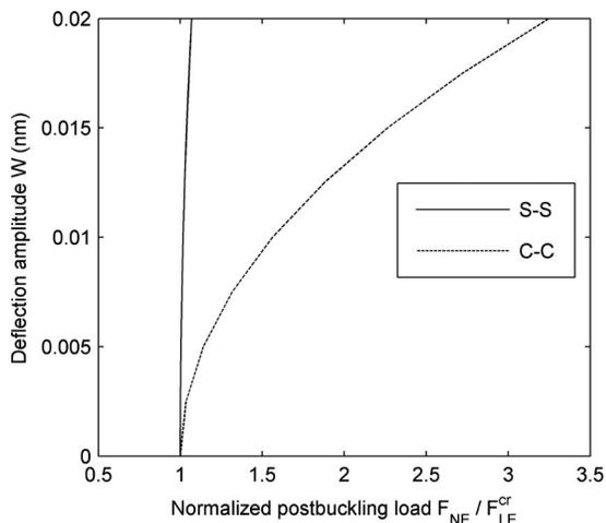
FIG. 6. Postbuckling behavior of an embedded CNT with different end conditions ( $d=0.7$  nm and  $L=20d$ ).
