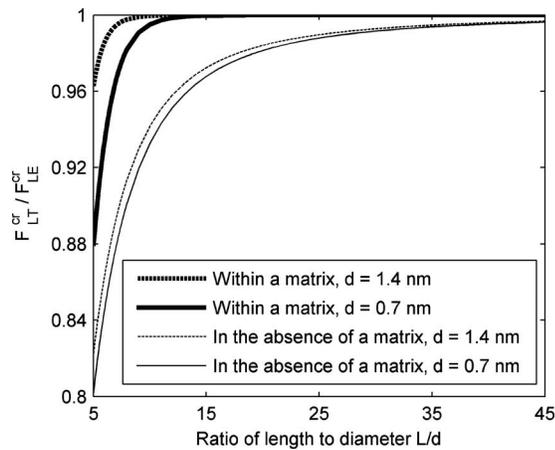
FIG. 9. Variation in the critical buckling load of an embedded CNT with  $L/d$  ( $d=0.7$  nm).
