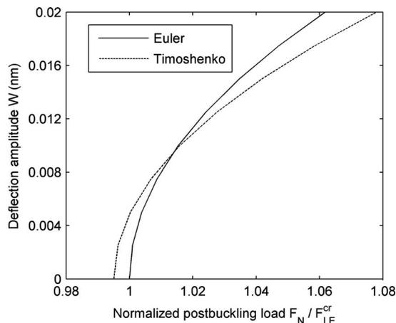
FIG. 7. Postbuckling behavior of an embedded CNT using different beam models with S-S end condition ( $d=0.7$  nm and  $L=10d$ ).
