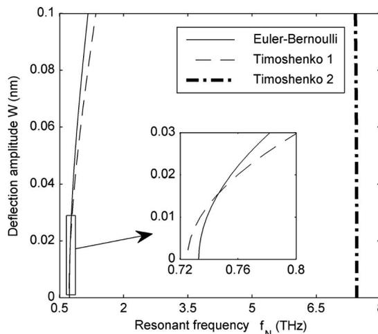
FIG. 4. Vibrational mode of an embedded CNT for different beam models with S-S end condition ( $d=0.7$  nm and  $L=10d$ ).
