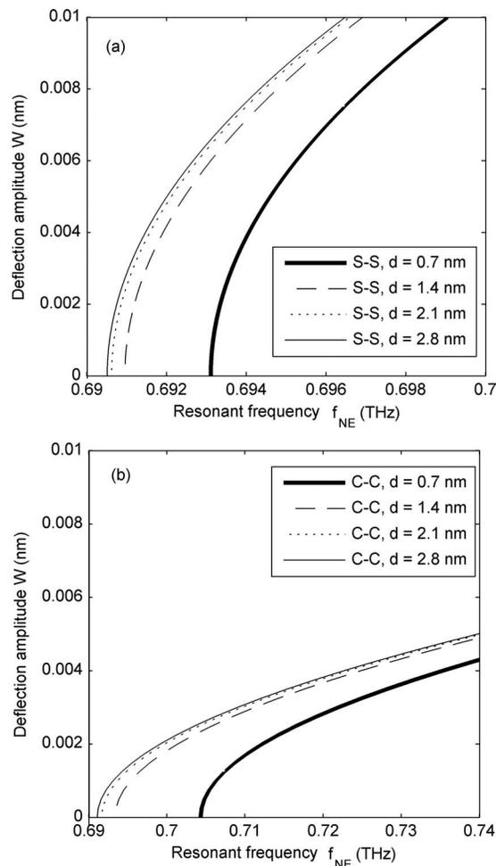
FIG. 2. CNT size effect on the resonant frequencies of an embedded CNT with (a) S-S and (b) C-C end conditions ( $L=20d$ ).
