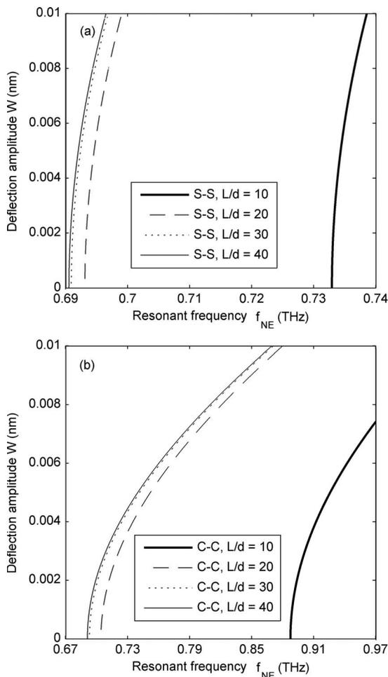
FIG. 3. Effect of CNT length-to-diameter ratio on the resonant frequencies of an embedded CNT with (a) S-S and (b) C-C end conditions ( $d=0.7$  nm).
