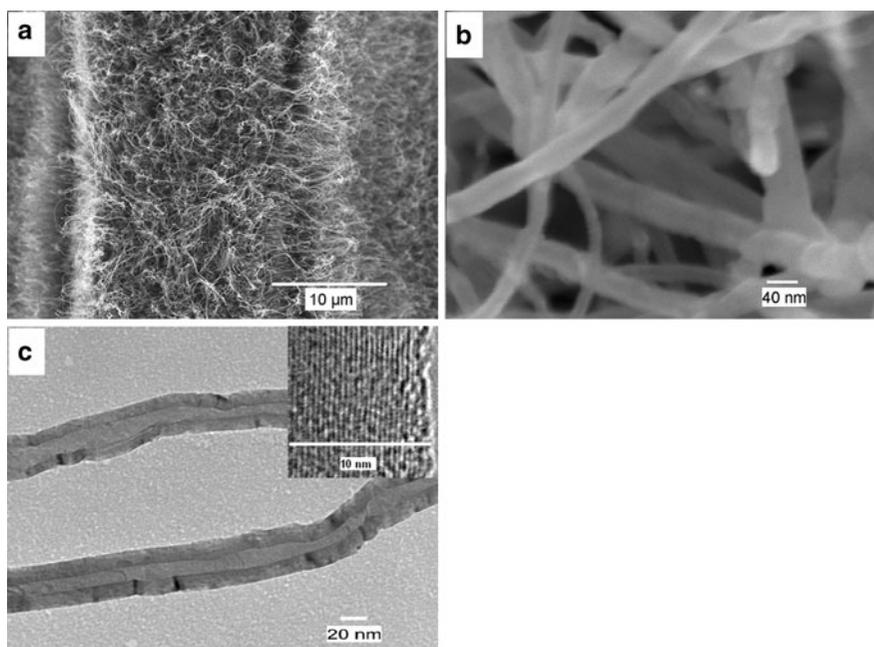
**Fig. 2** 200-cycle ALD of iron oxide deposition on the undoped CNTs: without surface pretreatment, **a** SEM image and **b** TEM image; treated by 2 h nitric acid, **c** low magnification and **d** high magnification SEM image; treated by 2 h SDS, **e** low magnification and **f** high magnification SEM image; treated by 1 h nitric acid and 1 h SDS in sequence, **g** low magnification and **h** high magnification SEM image
