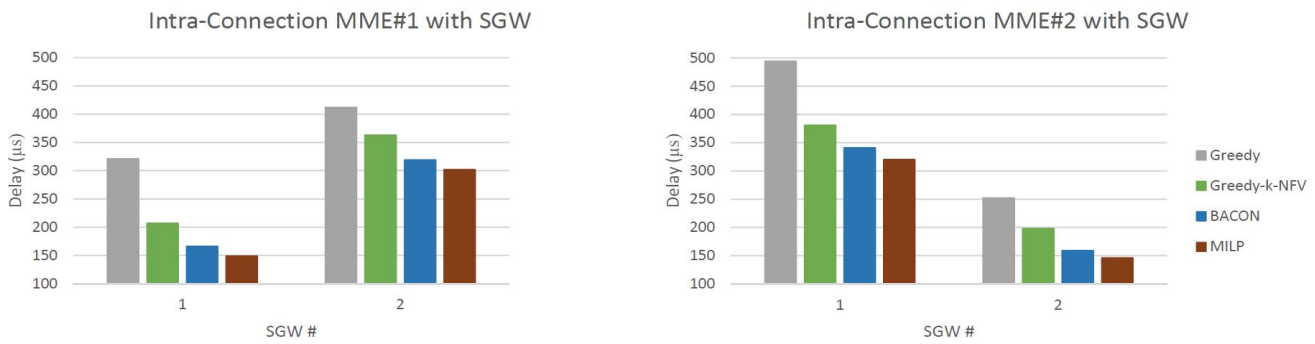
Fig. 4. Intra-connection delay between VNF instances of types MME and SGW.
