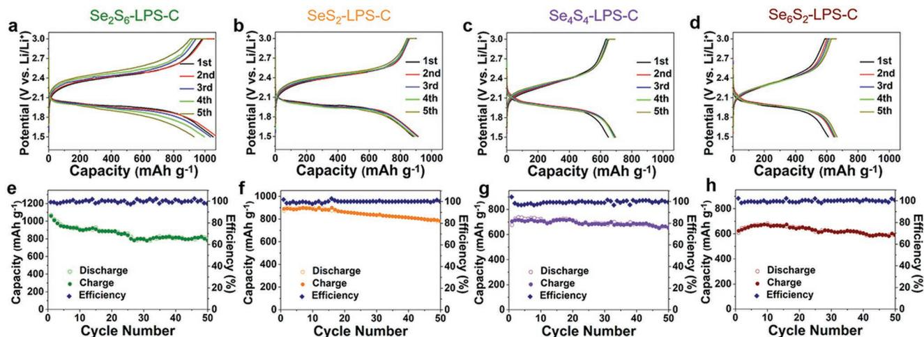
**Figure 3.** Electrochemical performance of  $\text{SeS}_x\text{-LPS-C}$  cathodes at 25 °C. a–d) Discharge–charge curves of cells with: a)  $\text{Se}_2\text{S}_6\text{-LPS-C}$ , b)  $\text{SeS}_2\text{-LPS-C}$ , c)  $\text{Se}_4\text{S}_4\text{-LPS-C}$ , and d)  $\text{Se}_6\text{S}_2\text{-LPS-C}$  cathodes at 50 mA  $\text{g}^{-1}$ . e–h) Cycling performance and Coulombic efficiencies of the  $\text{SeS}_x\text{-LPS-C}$  cathodes at 25 °C.
