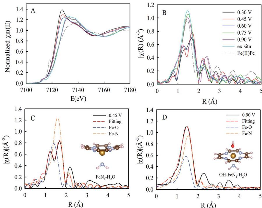
Fig. 8 XANES results of iron phthalocyanine (FePc) and C-FeHZ8@g-C<sub>3</sub>N<sub>4</sub>-950 (A); Fourier-transformed K-edge EXAFS of Fe for iron phthalocyanine (FePc) and C-FeHZ8@g-C<sub>3</sub>N<sub>4</sub>-950 (B); the EXAFS fitting result of C-FeHZ8@g-C<sub>3</sub>N<sub>4</sub>-950 at 0.45 V (C), and the EXAFS fitting result of C-FeHZ8@g-C<sub>3</sub>N<sub>4</sub>-950 at 0.90 V (D).
