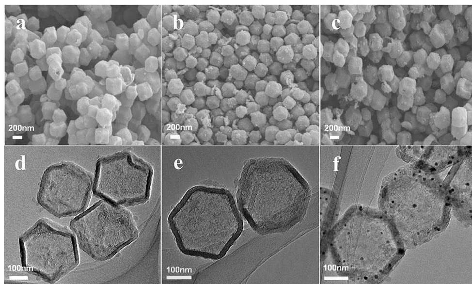
Fig. 1 SEM images of (a) C-HZ8-950, (b) C-FeHZ8@g-C<sub>3</sub>N<sub>4</sub>-950, and (c) C-FeHZ8-950; TEM images of (d) C-HZ8-950, (e) C-FeHZ8@g-C<sub>3</sub>N<sub>4</sub>-950, and (f) C-FeHZ8-950.
