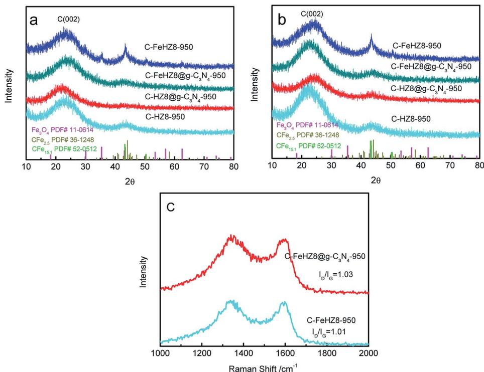
Fig. 3 XRD patterns of C-HZ8-950, C-HZ8@g-C<sub>3</sub>N<sub>4</sub>-950, C-FeHZ8-950, and C-FeHZ8@g-C<sub>3</sub>N<sub>4</sub>-950 (a) before acid leaching and (b) after acid leaching; (c) Raman spectra of C-FeHZ8-950 and C-FeHZ8@g-C<sub>3</sub>N<sub>4</sub>-950.
