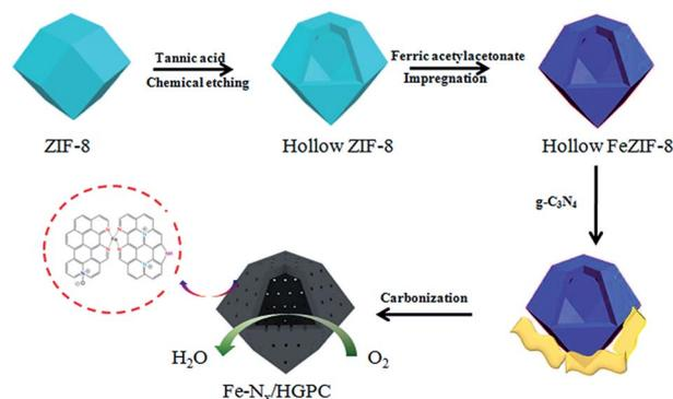
Scheme 1 Schematic illustration of the C-FeHZ8@g-C<sub>3</sub>N<sub>4</sub>-950 synthesis.
