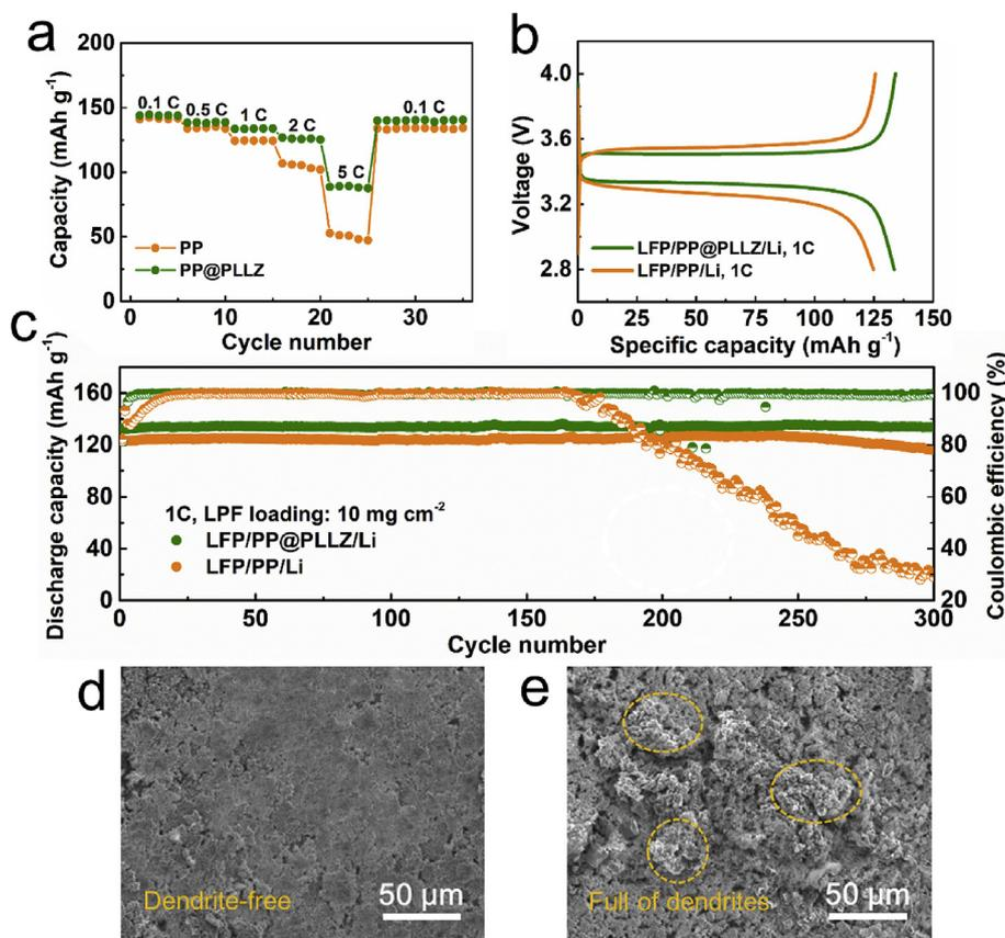
**Fig. 4.** a) Rate performance of LFP/Li cells with different separators. b) Charge/discharge curves and c) cycle performance of LFP/Li cells with different separators at 1C (1C = 170 mA g<sup>-1</sup>). SEM images of Li metal anodes after cycling with d) PP@PLLZ separator and e) PP separator.
