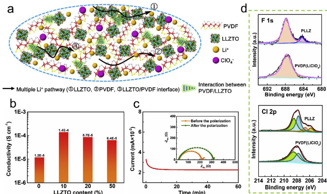
Fig. 3. a) Schematic illustration of multiple highly-conductive  $\text{Li}^+$  transportation pathways in the PLLZ layer. b) Ionic conductivities of PLLZ layers with different LLZTO contents. c)  $t_+$  of PLLZ (10%) layer. d) XPS spectra of F 1s and Cl 2p in PLLZ (10%) layer.
