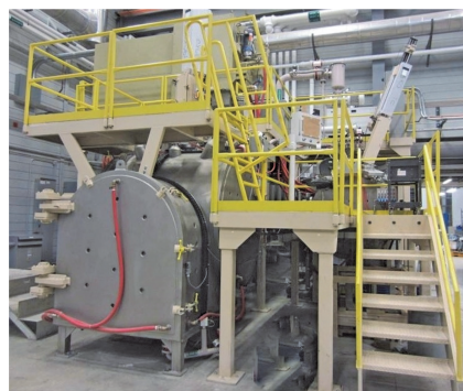
Fig. 6 — Vacuum induction furnace setup in a pilot-scale casting laboratory at Canmet-Materials.
