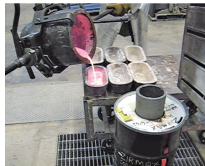
Fig. 7 — Pouring LFP melt at approximately 1000°C into 5-kg ingot molds.
