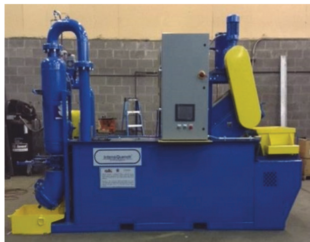
Fig. 1 — Portable 600-gallon DFIQ system (patent pending) for quenching forgings.
