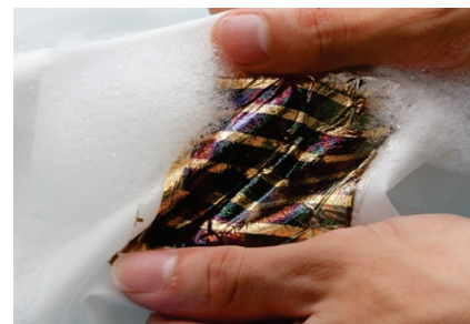
Washable, ultra-thin organic solar cells.
