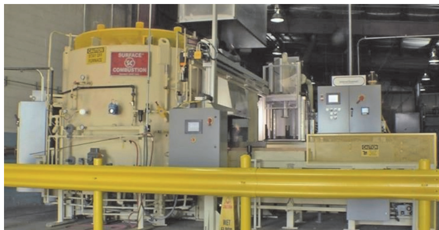
Fig. 4 — Fully automated, single-part processing IntensiQuench system for hardening gears.
