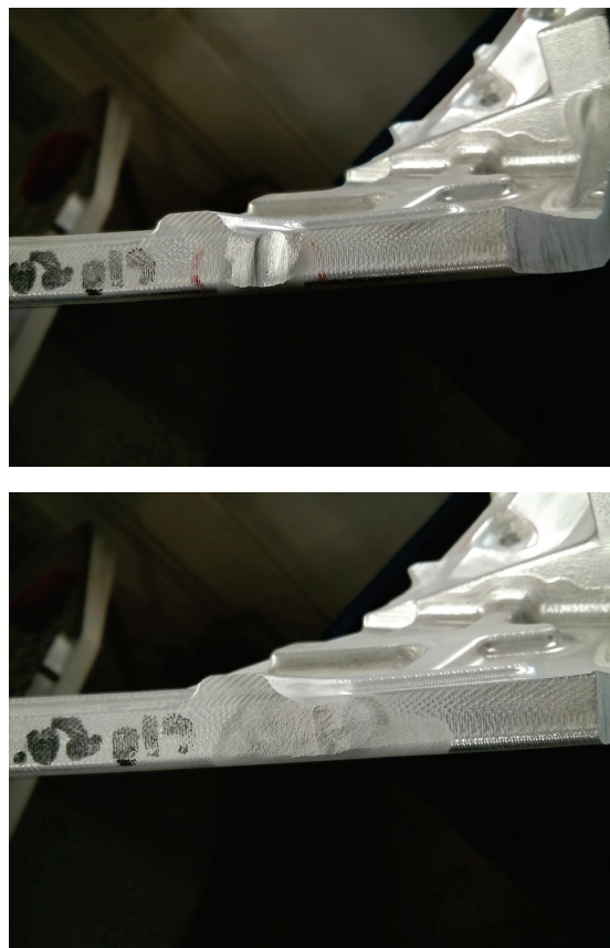
Fig. 5 — Snap-off defect dimensionally repaired with SST cold spray, before (top) and after (bottom).
