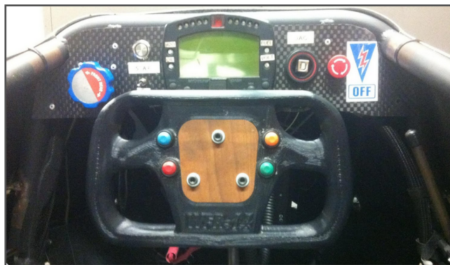
3D printed, custom molded Steering Wheel
