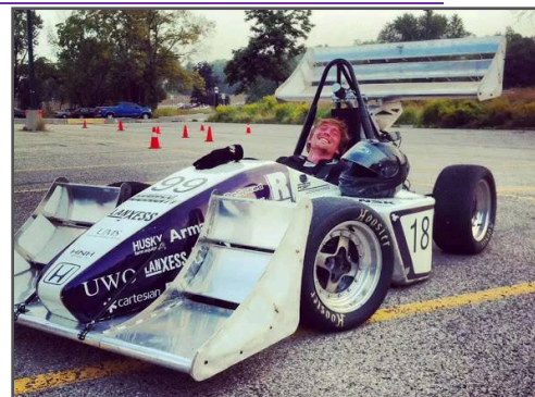
Ryan Alexander with prototyped aluminum wings on the 2013 car
