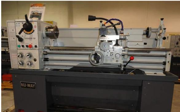
**Potential Hazards:** High power rotating spindle with exposed moving parts can cause entanglement, impact, flying debris and electrical hazard with the potential to cause serious harm and/or even death. Exposure to heat, noise, projectiles and sharp objects.
