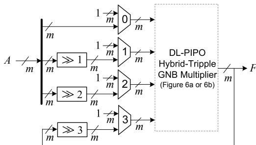
Figure 8: Architecture of the proposed eight-ary field exponentiation scheme. The 1 inputs to multiplexers represent the field element  $1 = (1, \dots, 1)$  represented in the GNB.
