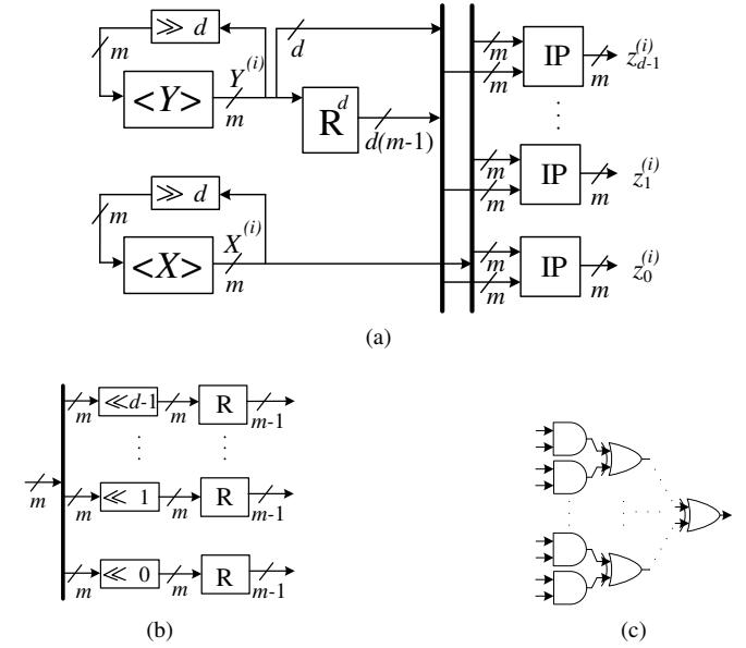
Figure 4: (a) The proposed architecture of the MSD DL-PISO single GNB multiplier. (b) Architecture of the  $R^d$  block before applying sub-expression sharing. (c) Architecture of the IP block.  $0 \leq i < k$  denotes the iteration number,  $k = \lceil \frac{m}{d} \rceil$ .
