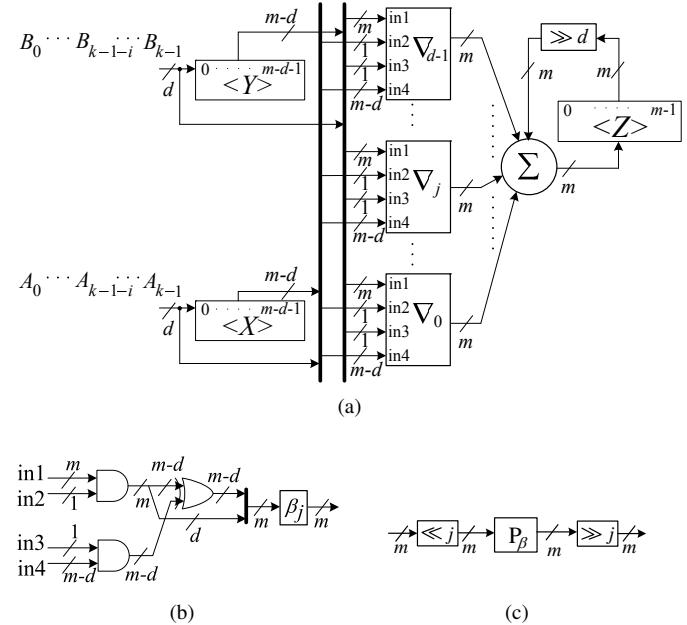
Figure 2: (a) Architecture of the proposed MSD DL-FSIPO single GNB multiplier. (b) Architecture of  $\nabla_j$ . (c) Architecture of  $\beta_j$ .
