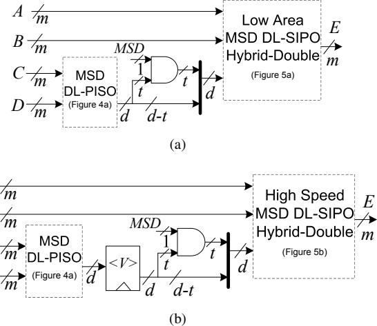
Figure 6: Architectures of the proposed DL-PIPO hybrid-triple GNB multiplier: (a) Low area design. (b) High speed design.
