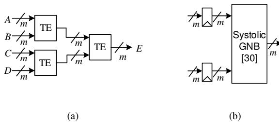
Figure 7: (a) Tree structured triple multiplier based on systolic GNB multiplier in [30]. (b) Tree element (TE).
