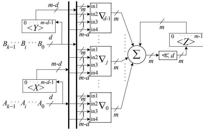
Figure 3: Architecture of the proposed LSD DL-FSIPo single GNB multiplier. Architecture of  $\nabla_j$  and  $\beta_j$  (which is a component of  $\nabla_j$ ) blocks are shown in Figures 2b and 2c, respectively, where in Figure 2b, and at iteration  $0 \leq i < k$ , we have:  $\text{in}1 = B_i + B^{(i-1)}$ ,  $\text{in}2 = a_{di+j-r}$ ,  $\text{in}3 = b_{di+j-r}$ , and  $\text{in}4 = A^{(i-1)}$ .
