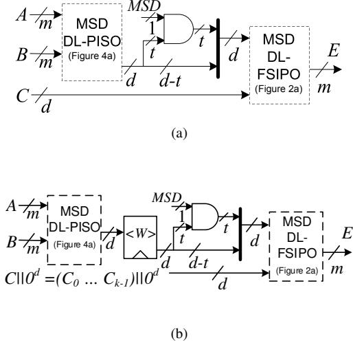
Figure 5: Architectures of the proposed MSD DL-SIPO hybrid-double GNB multiplier, where  $t = k \times d - m$ : (a) Low area design. (b) High speed design. The appended  $0^d$  (zero digit) in input  $C$  balances the timing due to pipelining.
