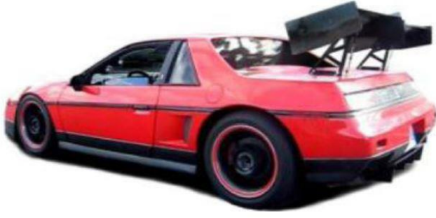
Figure 9. Physical prototype of active aerodynamic control system mounted on a vehicle [11].
