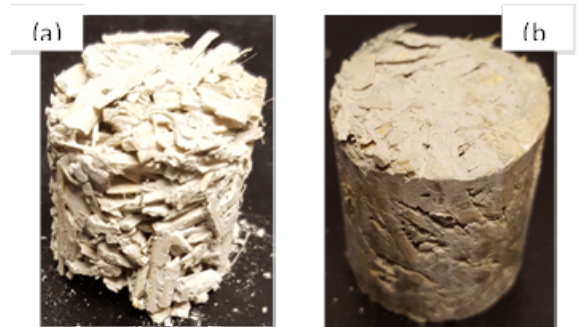
Fig.1: Example of low-density (a) and high-density (b) lime/concrete samples [3]
