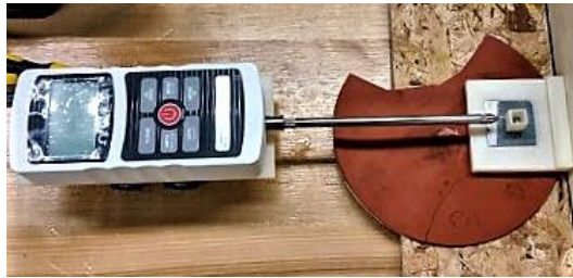
Figure 1 Experimental setup, (a) schematic of the system, also showing the way of ice formation on a test substrate, and (b) a picture showing the measurement
