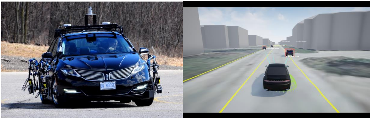
Figure 1 (Left): Autonomoose equipped with VMS to gather experimental data Figure 2 (Right): Autonomoose model in the Unreal environment
