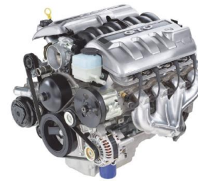
Figure 1. Car engine and its front end accessory drive belt transmission [2].
