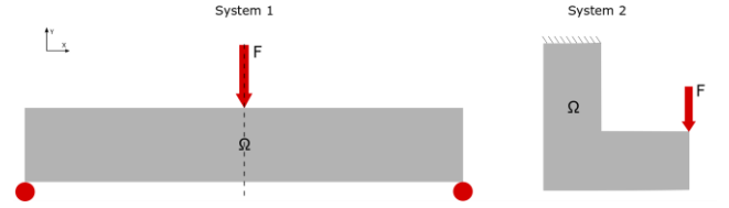
Figure 4 System 1: The MBB beam problem with a 6:1 length to width ratio and load F . The grey region \Omega will be taken as the design space for topology optimization, the two red circles show the supports. System 2: The L-Bracket problem with each arm being 200mm in length and 80mm in width.
