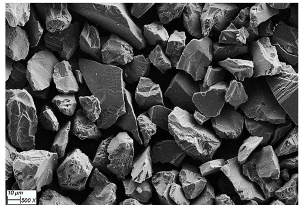
Figure 1. Morphology of the alumina powder used in FS process at 500X magnification.
