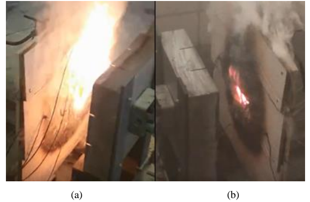
Figure 8. Comparison of the ignition process of the EW prototype under (a) the HHC and (b) the LHC.
