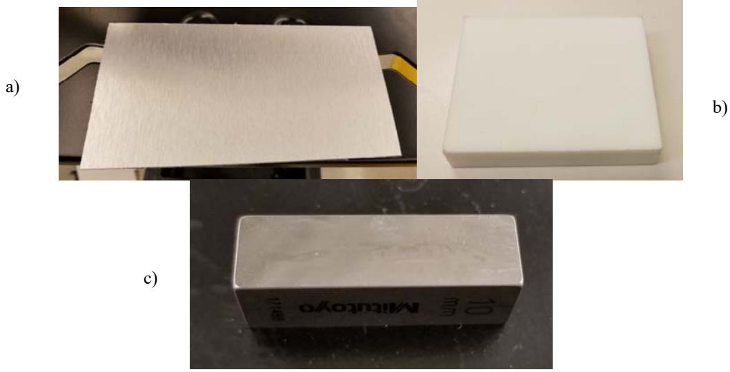
Figure 2. Test Samples a) Brushed Aluminum b) Selective Laser Sintered c) Gauge Block
