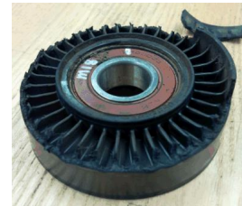
Figure 2. FRP structure failure due to overheating (Courtesy of Litens Automotive Group).
