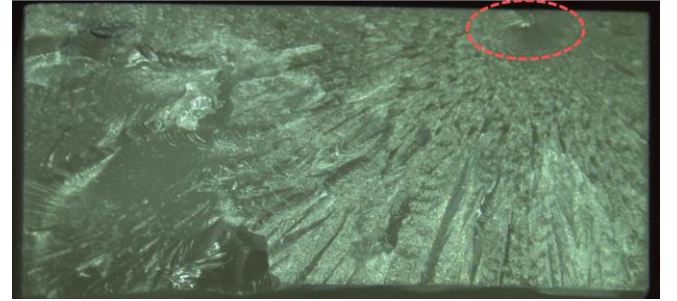
Figure 9. Fractured surface from specimen DB2 showing crazes of cracking.
