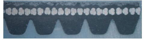
Figure 5. The Belt cross-section (Courtesy of Litens Automotive Group).
