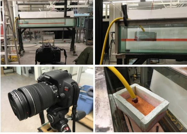
Figure 2. Laboratory equipment. Video recording camera (bottom left) and camera's position relative to tank (top left). Layering fresh water on top of salt water using the sponge float (top and bottom right.)
