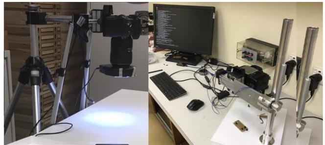
Figure 4 Camera set-up for photogrammetry analysis of the insect wings
