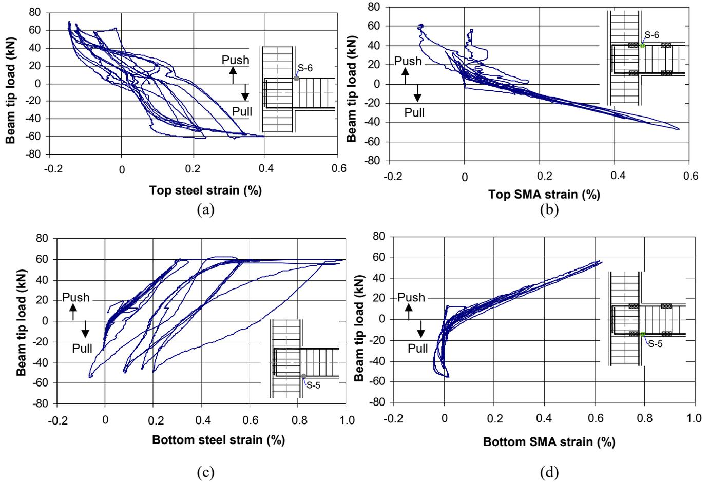
Fig. 14. Strains in main longitudinal reinforcements at the column face of joint specimens: (a) top rebar of JBC-1, (b) top rebar of JBC-2, (c) bottom rebar of JBC-1, and (d) bottom rebar of JBC-2.
