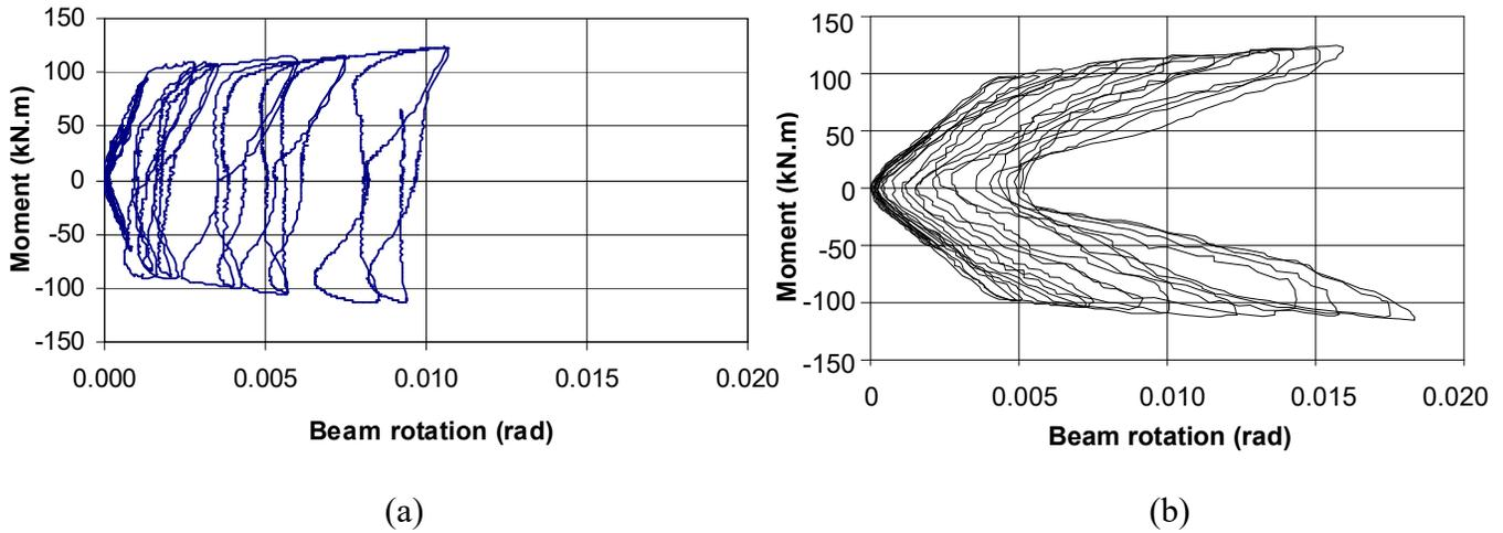
Fig. 12. Beam moment-rotation plots at 180mm away from the column face of specimens: (a) JBC-1, and (b) JBC-2.
