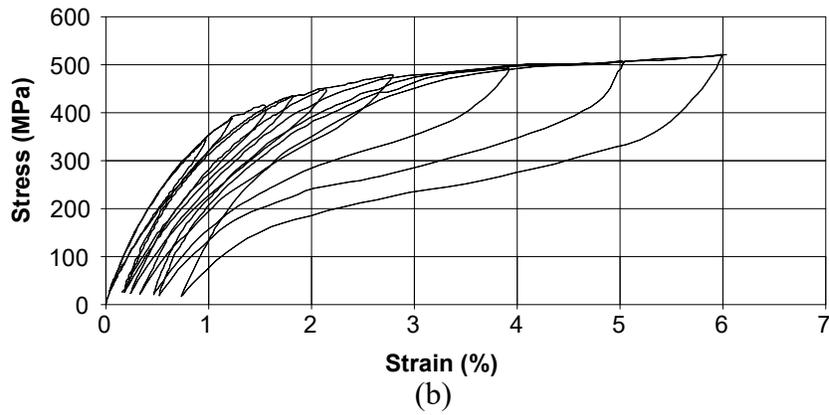
Fig. 5. (a) Typical stress-strain behaviour of SE SMA and steel; and (b) experimental cyclic tensile strength of SE SMA rebar within couplers.
