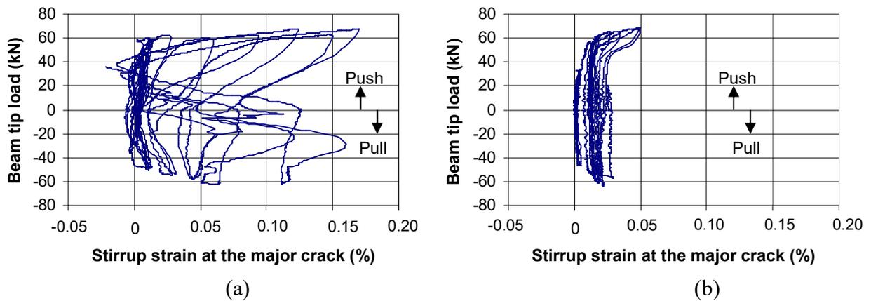
Fig. 15. Strains in transverse reinforcement at the location of major crack of specimens (a) JBC-1, and (b) JBC-2.
