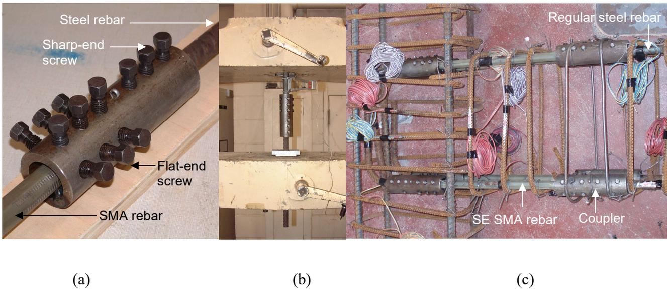
Fig. 4. (a) Coupler used in JBC-2, (b) test setup of coupler in universal testing machine, and (c) reinforcement caging of JBC-2.
