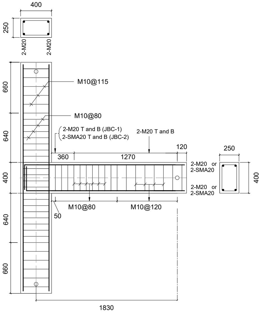
Fig. 2. Reinforcement details of specimens JBC-1 and JBC-2 (all dimensions in mm).
