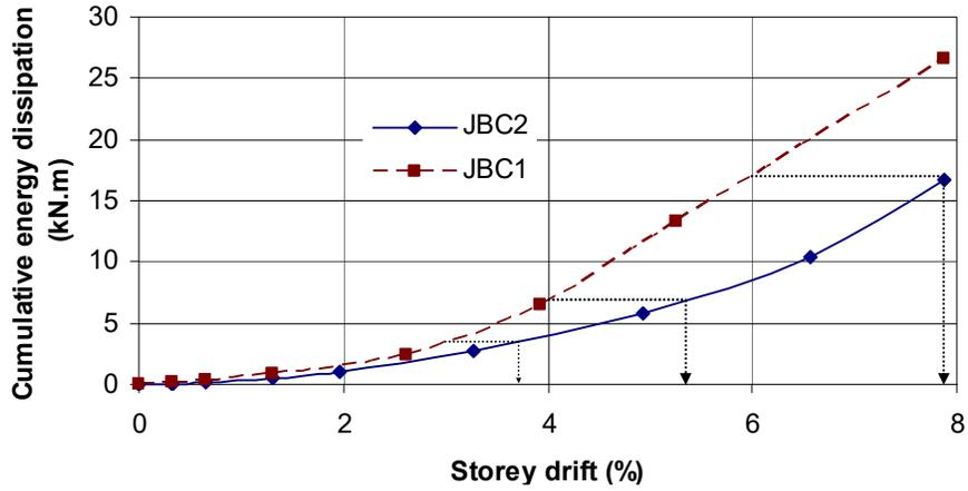
Fig. 11. Cumulative energy dissipation-storey drifts relationship of specimens JBC-1 and JBC-2.
