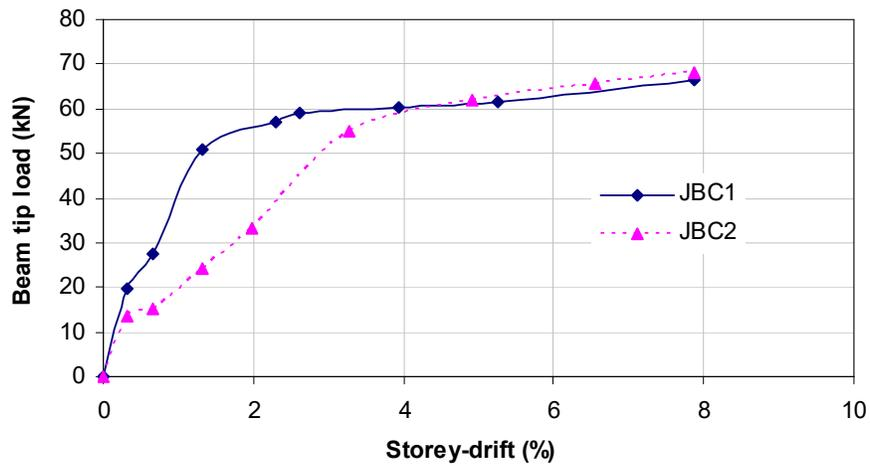
Fig. 10. Beam tip-load versus storey drift envelope of the tested specimens JBC-1 and JBC-2.
