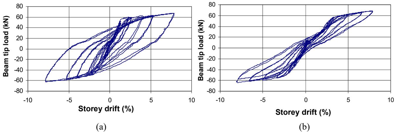
Fig. 8. Beam tip load-storey drift relationship of specimens: (a) JBC-1 and (b) JBC-2.
