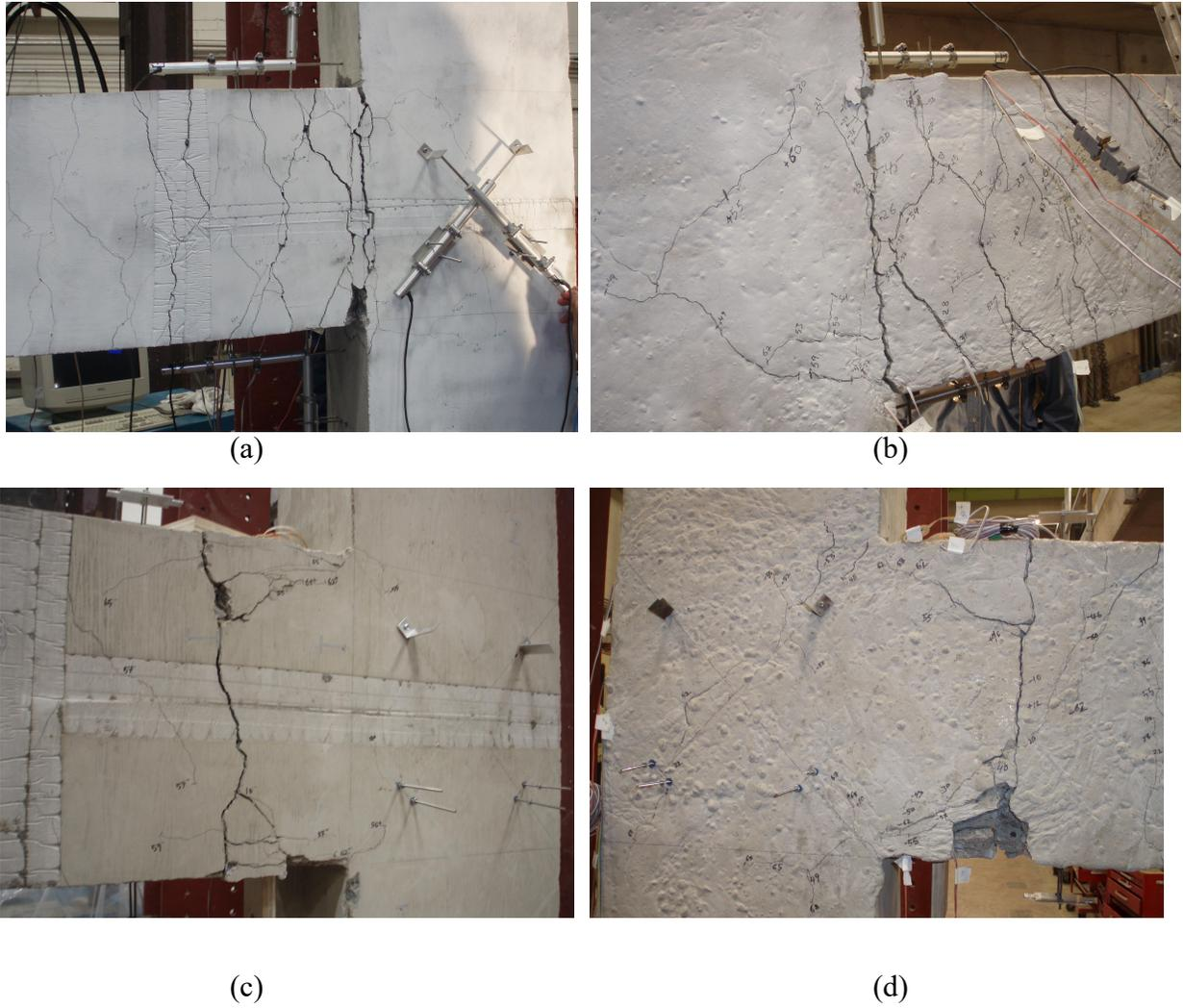
Fig. 9. Crack pattern of specimens after being subjected to cycles up to 72 mm: (a) front face of JBC-1, (b) rear face of JBC-1, (c) front face of JBC-2, and (d) rear face of JBC-2.
