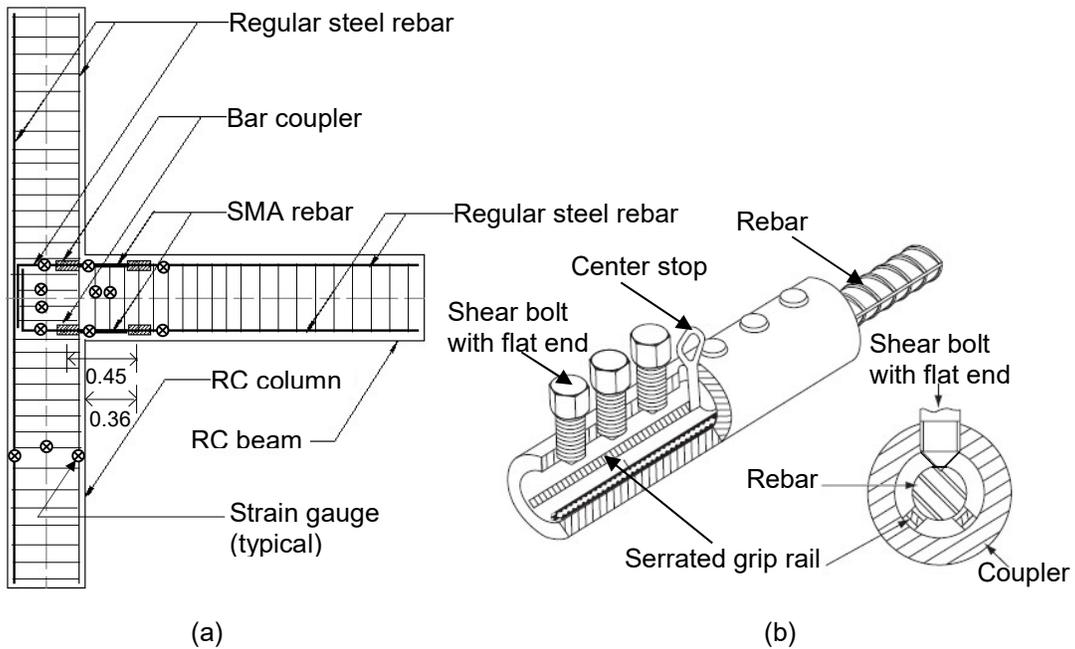
Fig. 3. (a) Splice details of specimen JBC-2 and the positions of strain gauges, (b) regular single barrel screw-lock coupler for connecting SMA rebar with regular steel rebar (all dimensions in m).
