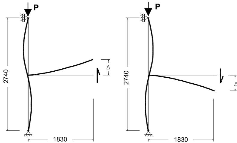
Fig. 6. Typical deflected shape of specimen under reversed cycle of beam tip displacement.
