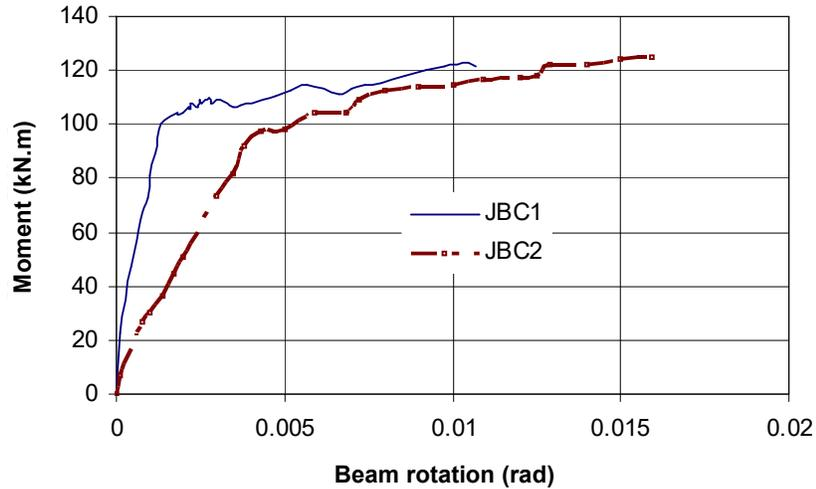
Fig. 13. Beam moment versus rotation envelope of the tested specimens.
