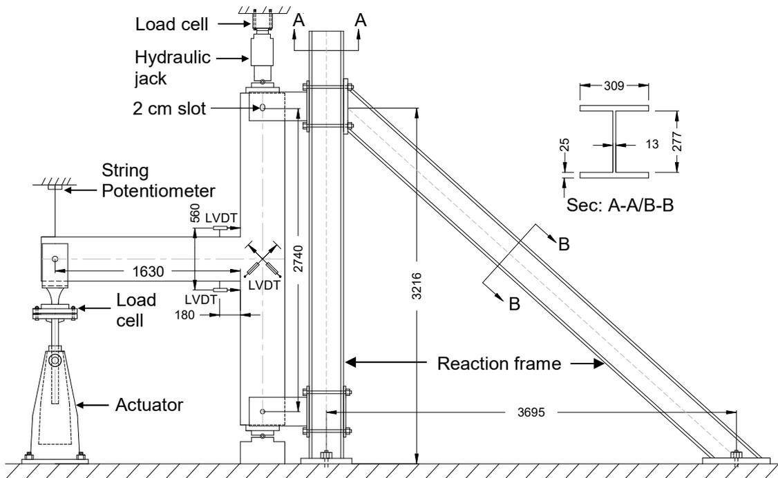
Fig. 7. Test setup (all dimensions in mm).
