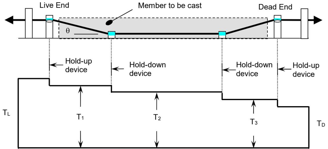
Figure 2: Strand Tension Force Distribution from Live End to Dead End.
