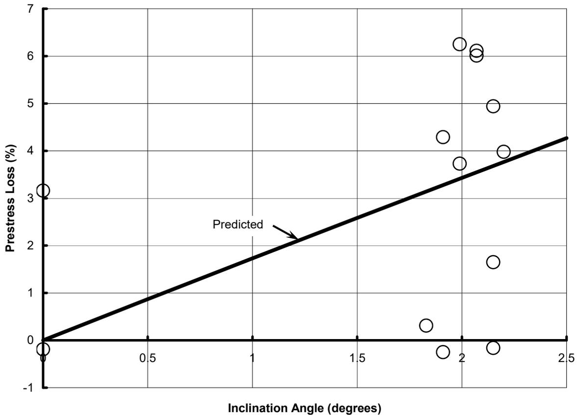
Figure 6: Prestress Loss versus Inclination Angle
