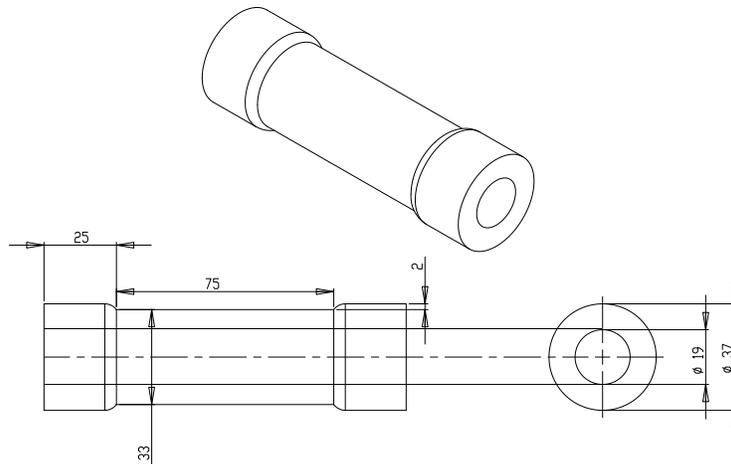
Figure 3: Shop Drawing of Load Cell
