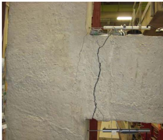
**Fig. 6:** Crack pattern of specimen JBC-4 after being subjected to reversed cyclic loading.
