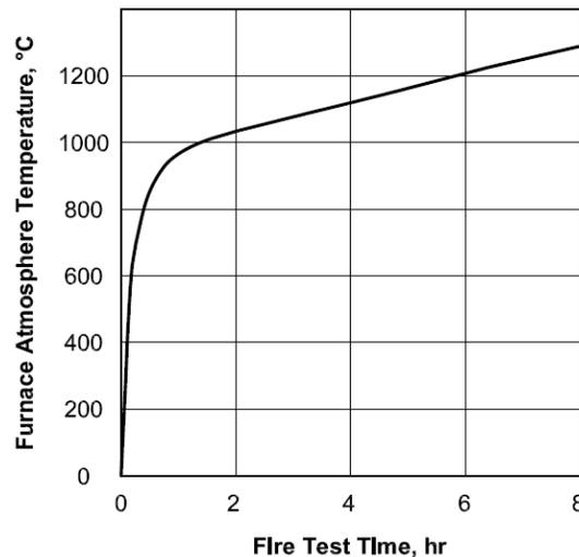
**Figure 3: ASTM E119 Standard Fire Curve (ACI 216R-89 1989)**
