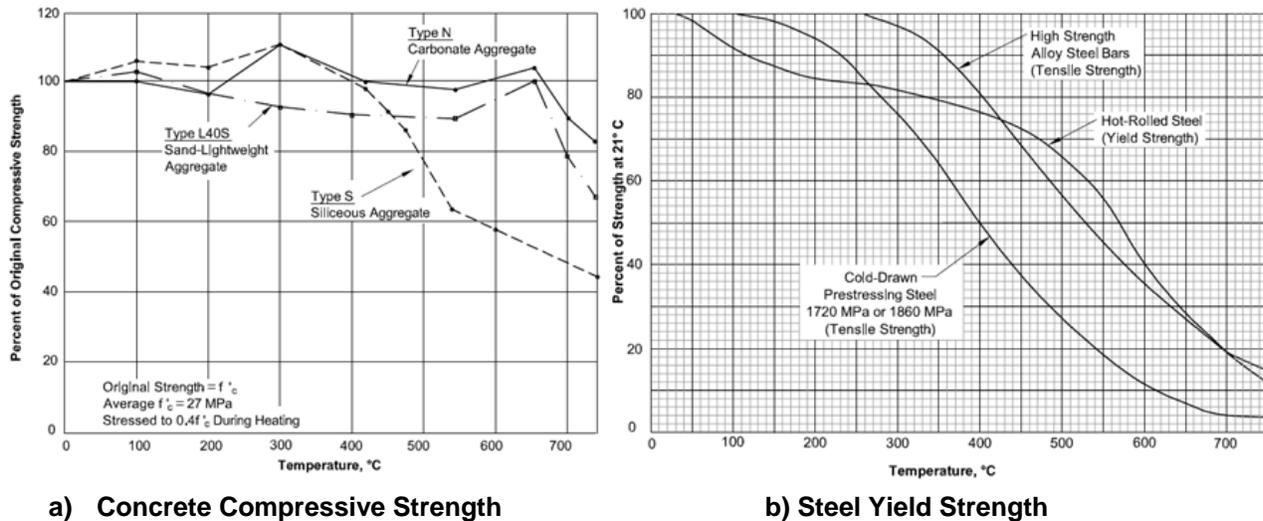
**Figure 1: Effect of Elevated Temperatures on Reinforced Concrete Materials (CPCI 2007)**
