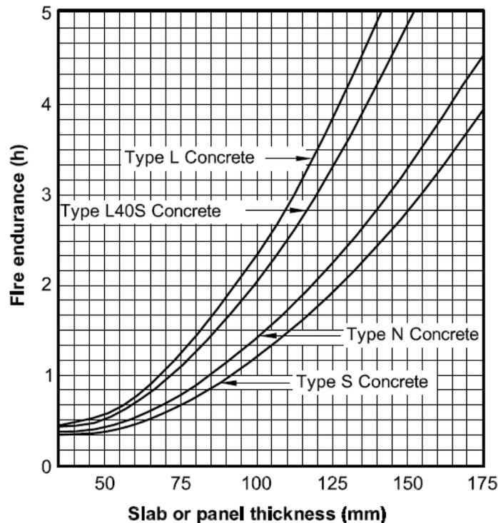
Figure 4: Chart for Determining Fire Resistance of Walls (CPCI Design Manual 2007)
