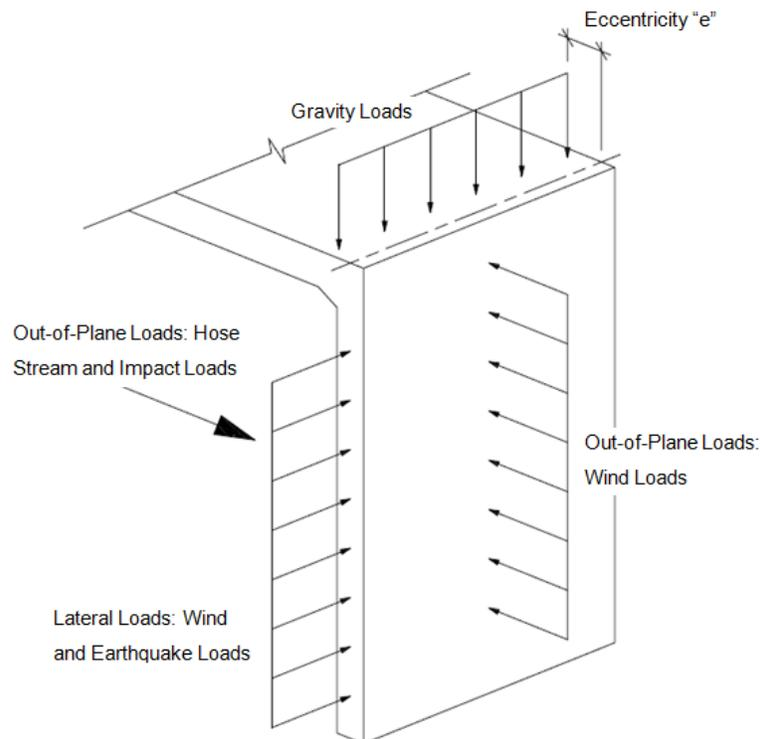
Figure 2: Loads Resisted by Concrete Walls
