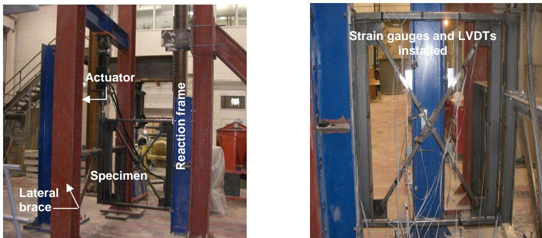
Figure 3. Schematic Representation and Overall View of Test Setup
