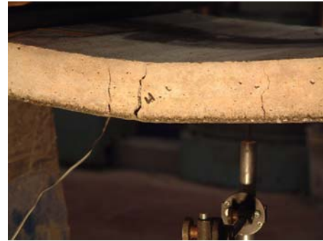
b) crack pattern (side view of the slab)
