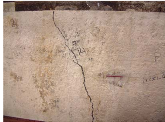
b) crack pattern (bottom view of the slab)
