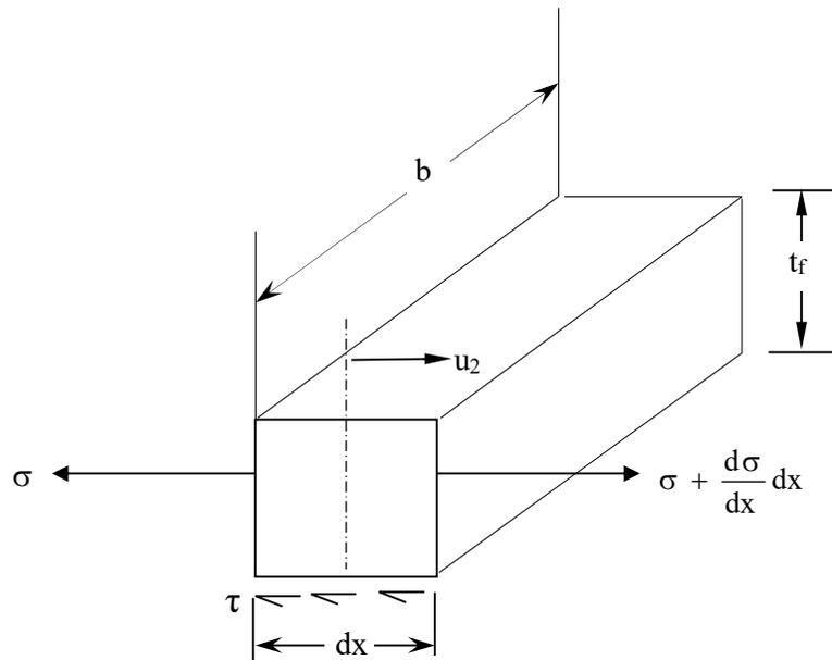
Figure 3a Stresses Acting on an Infinitesimal Element (dx) of the GFRP Plate
