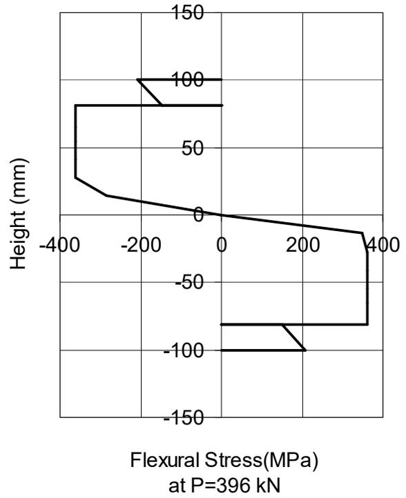
Figure 8 Flexural Stresses at Mid-Span Section of Rehabilitated Beam
