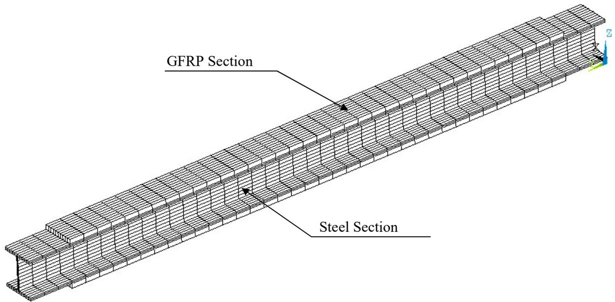
Figure 4 Typical Finite Element Mesh for the Rehabilitated Beam
