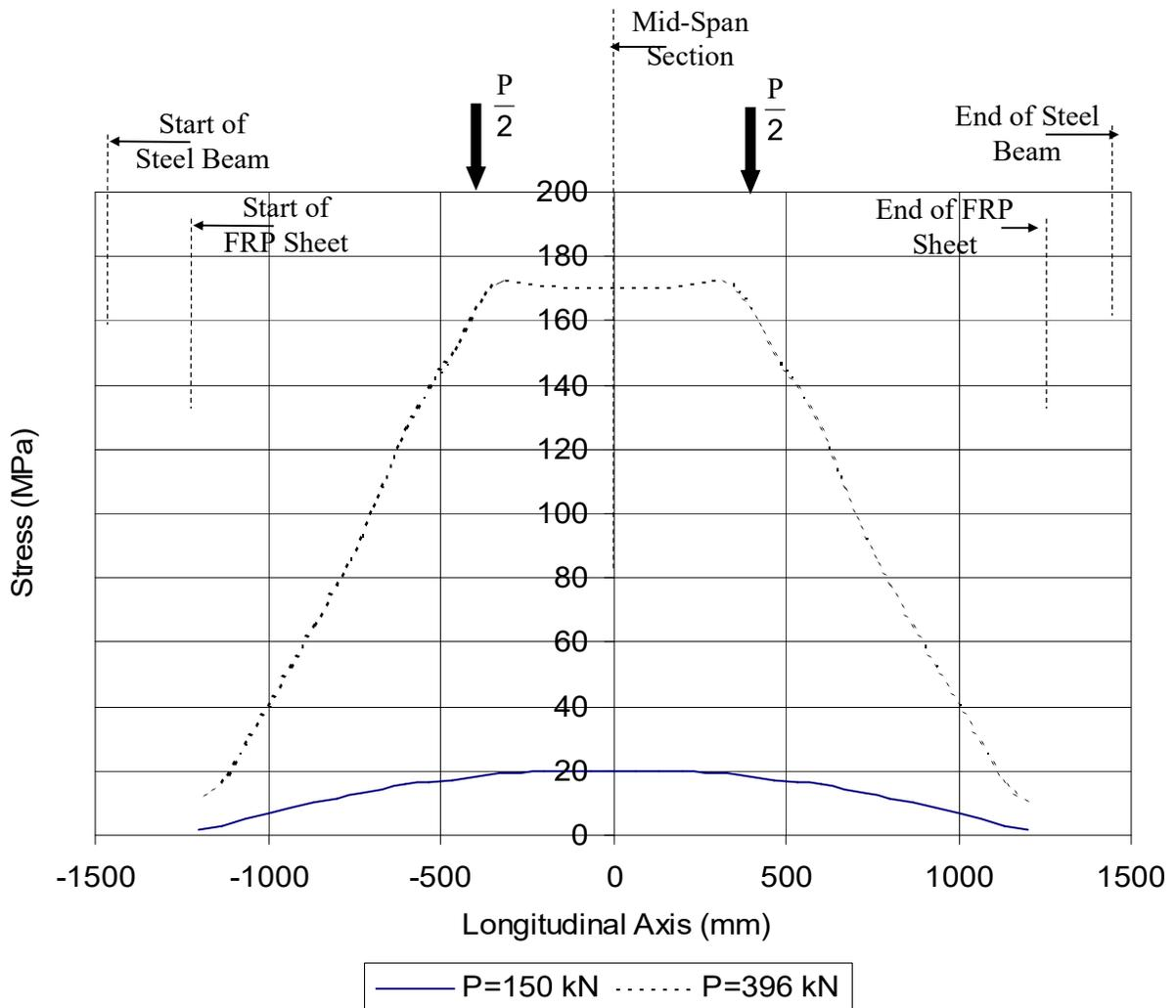
Figure 12 Bottom GFRP Sheet Longitudinal Axial Stress Distribution
