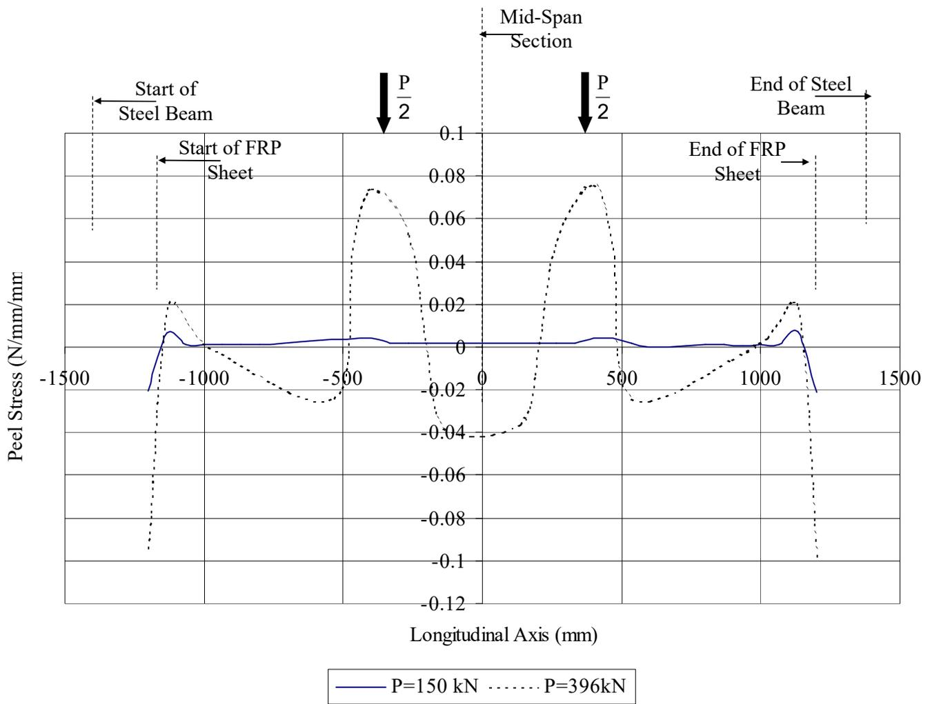
Figure 11 Longitudinal Peel-Stress Distribution for the Adhesive Connecting the Bottom Flange and the GFRP Sheet
