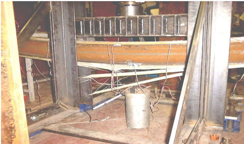
Figure 6 Failure of Rehabilitated Steel Beam
