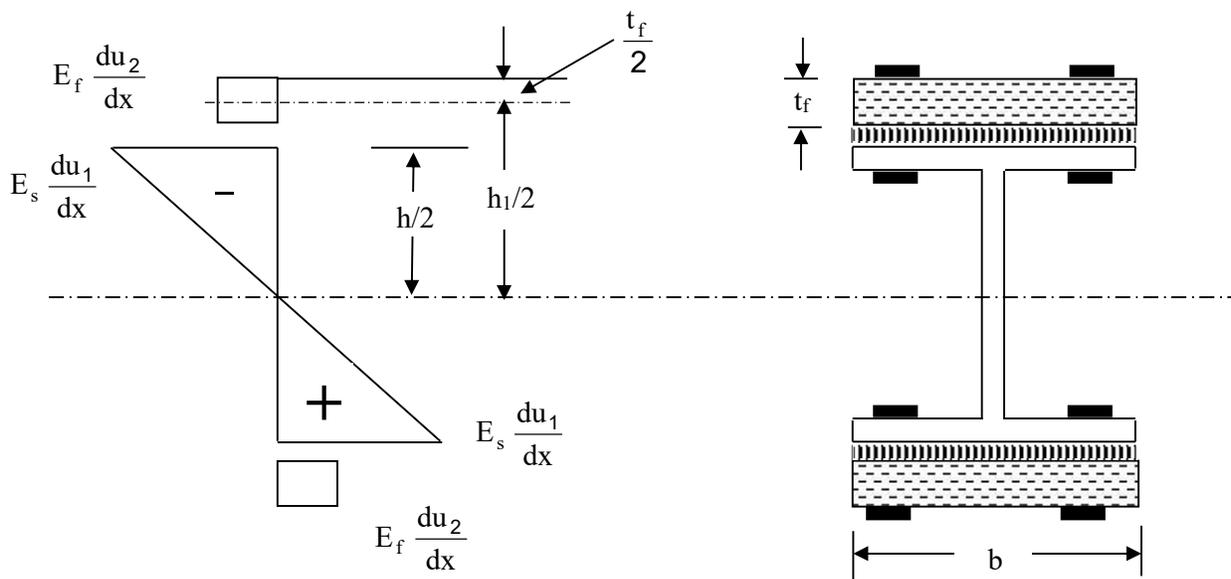
Figure 3b Typical Distribution of Axial Stress along the Depth of the Steel/ GFRP Section
