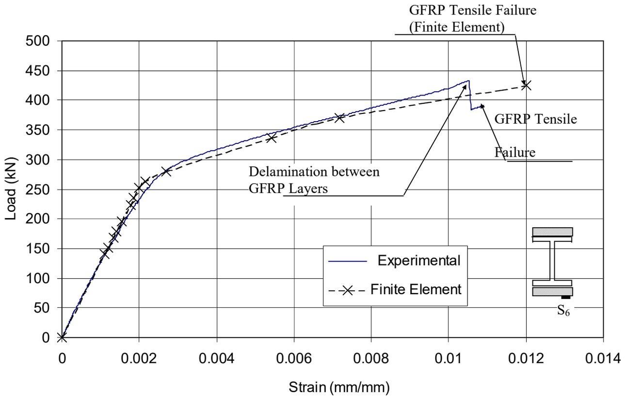
Figure 7a Rehabilitated Beam (B2): Load Strain Relationship Recorded by Strain Gauge S<sub>6</sub>
