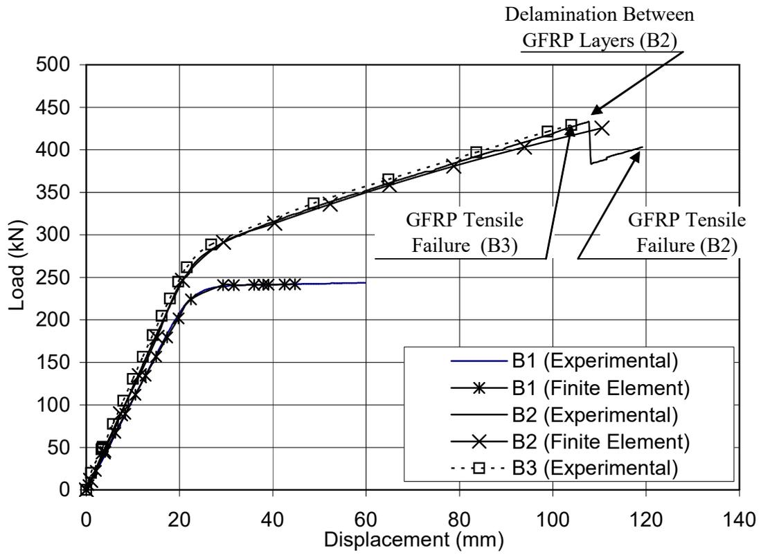
Figure 5 Load- Displacement Curve
