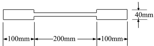
Figure 2c Steel Coupon Dimensions
