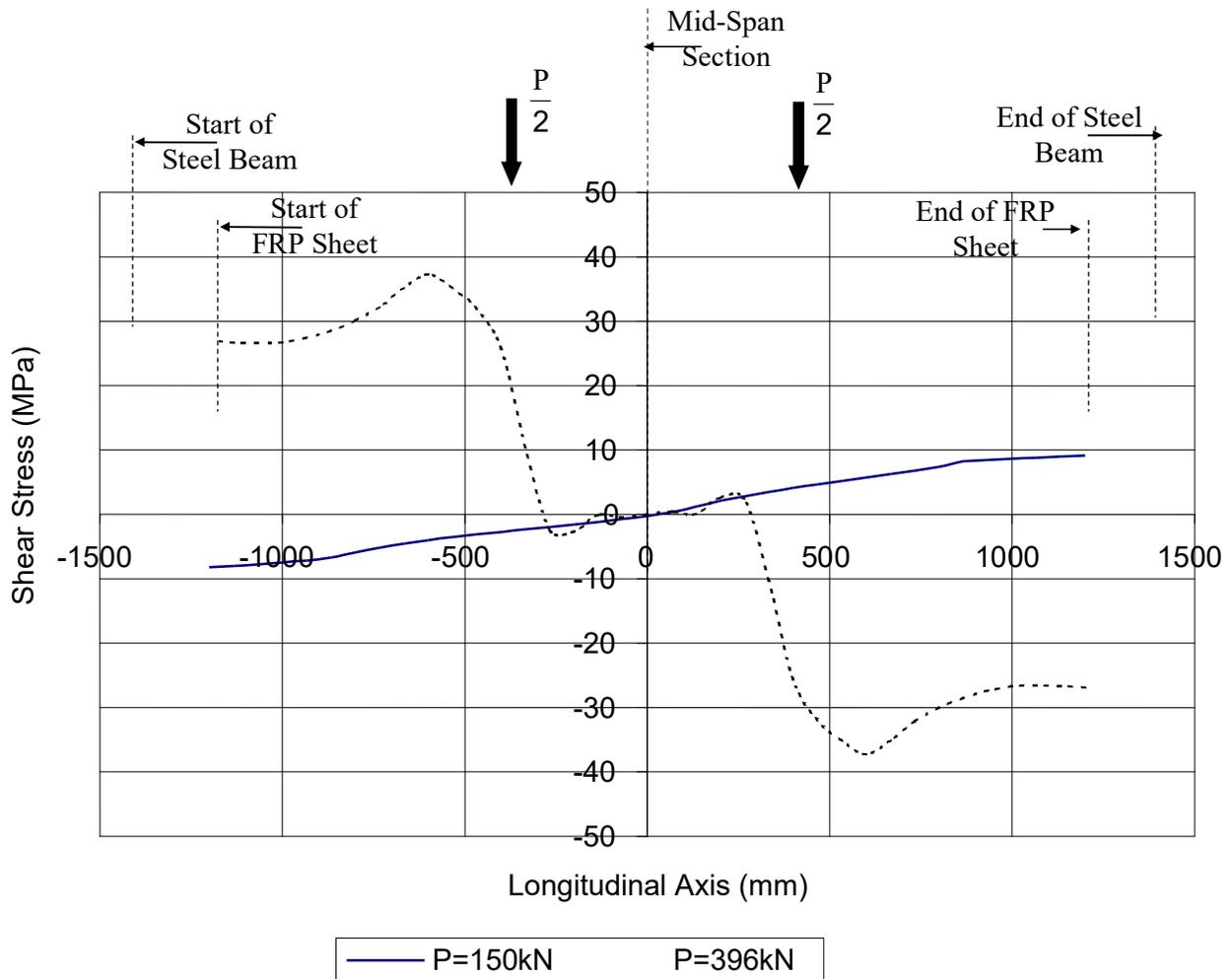
Figure 10 Longitudinal Shear-Stress Distribution for the Adhesive Connecting the Bottom Flange and the GFRP Sheet
