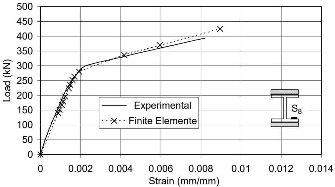
Figure 7b Rehabilitated Beam (B2): Load-Strain Relationship Recorded by Strain gauge S<sub>8</sub>
