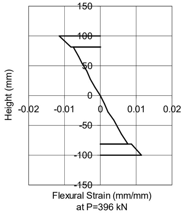
Figure 9 Flexural Stains at Mid-Span of Rehabilitated Beam
