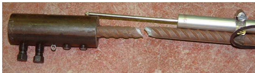
Figure 5. Failure pattern of 15M rebar in SBC coupler.
