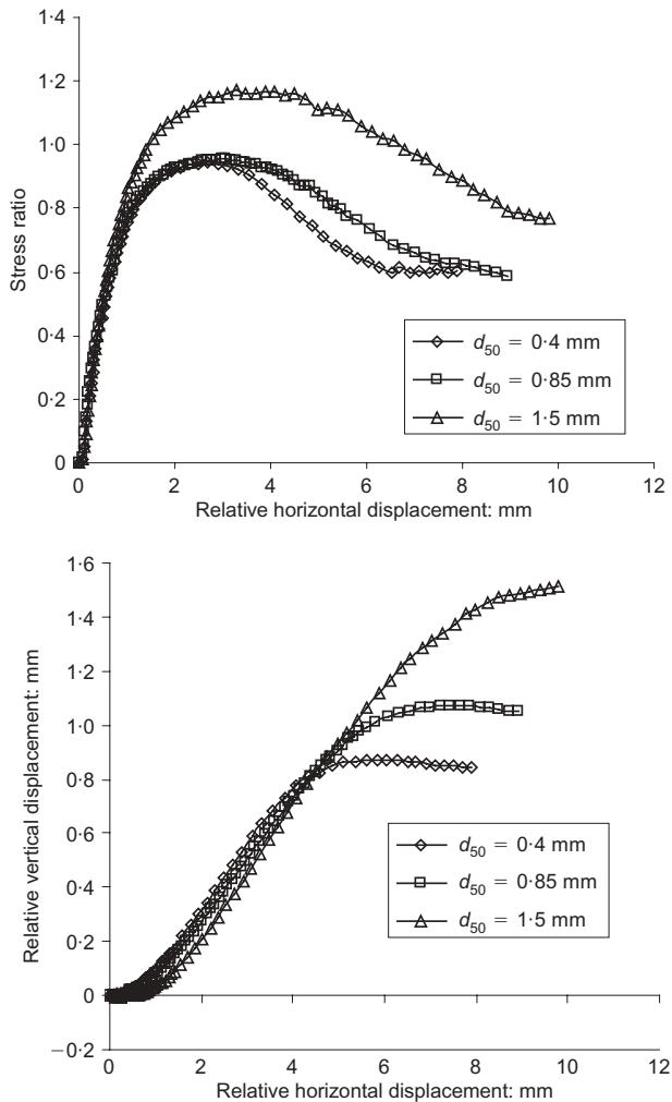
Fig. 10. Typical shear box tests on dense sands of different uniform gradings (characterised by  $d_{50}$  value) but at same initial void ratio and normal stress (3.2 kPa) (from Stone, 1988)
