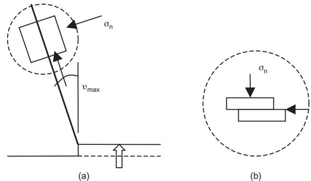
**Fig. 9. (a) Schematic representation of shear band propagating through dense cohesionless soil from induced boundary displacement; (b) direct shear analogue of shear band**
