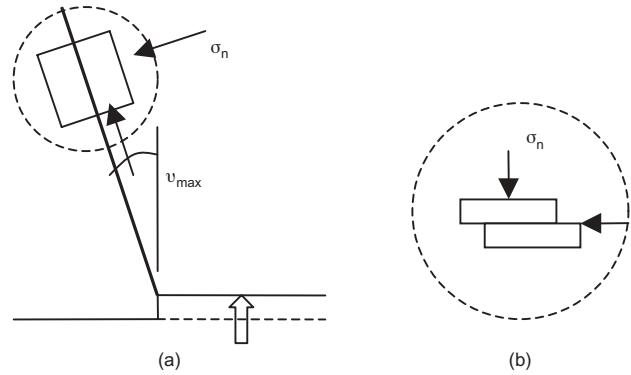
**Fig. 9.** (a) Schematic representation of shear band propagating through dense cohesionless soil from induced boundary displacement; (b) direct shear analogue of shear band
