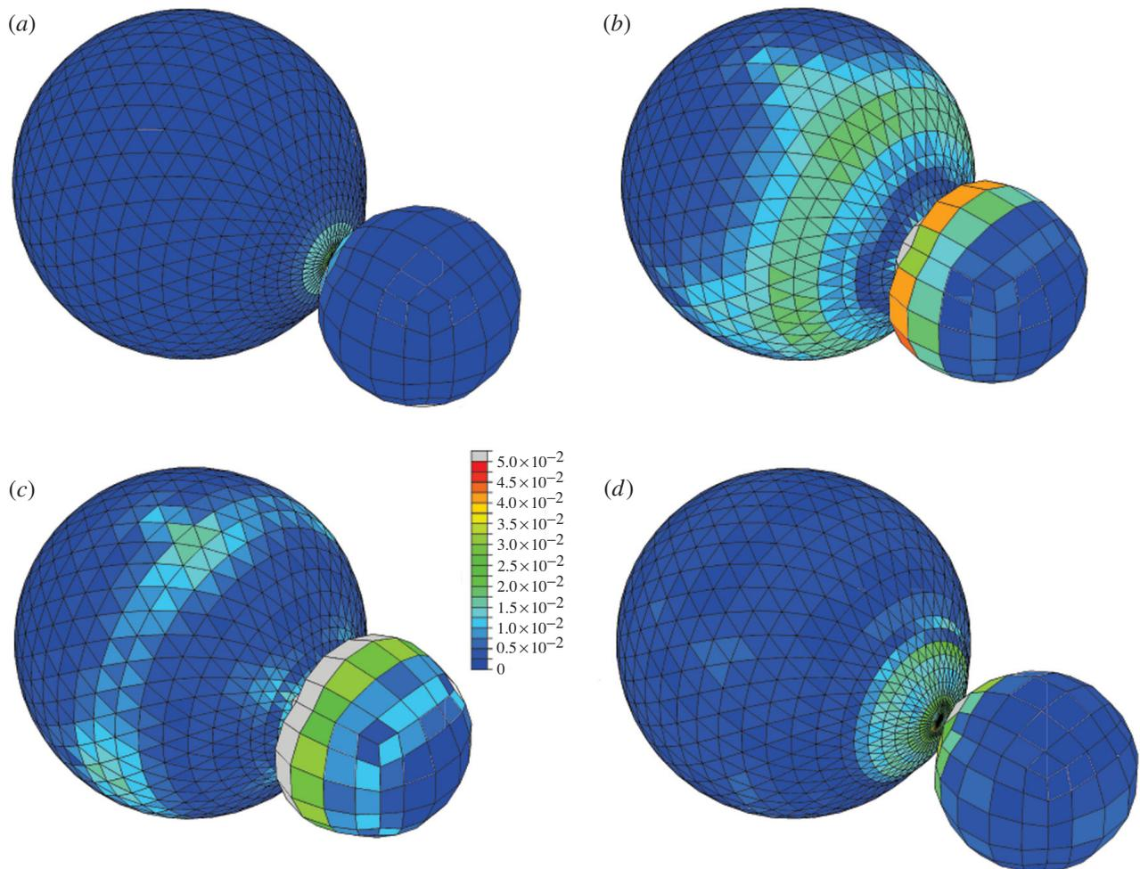
Figure 20. The pressure wave travelling through the eye in dynamic tonometry (units are  $\text{N mm}^{-2}$ ): (a) initial contact; (b) pressure wave; (c) dispersion of pressure wave; (d) pressure wave back at cornea following impact.
