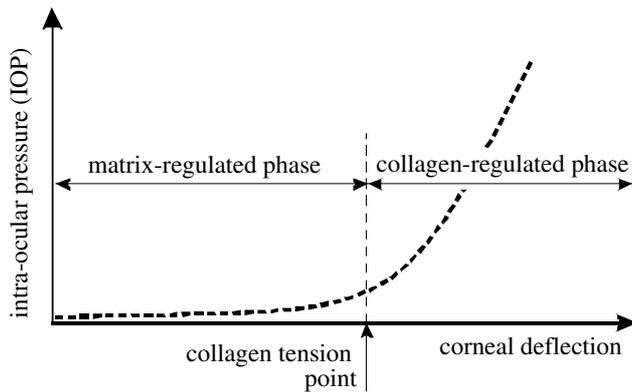
Figure 5. Corneal behaviour with an initial matrix regulated phase followed by a higher stiffness collagen regulated phase.
