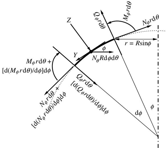
Figure 7. Straining actions acting in the meridian direction.
