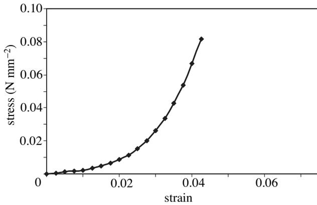
Figure 9. The average stress–strain relationship obtained from the trephinate inflation tests.
