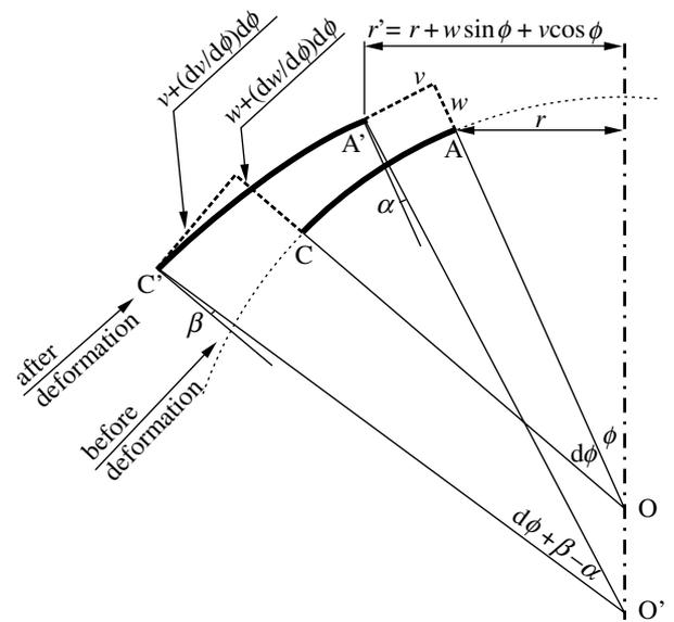
Figure 8. Displacements and rotations in the  $Y$ - $Z$  plane.
