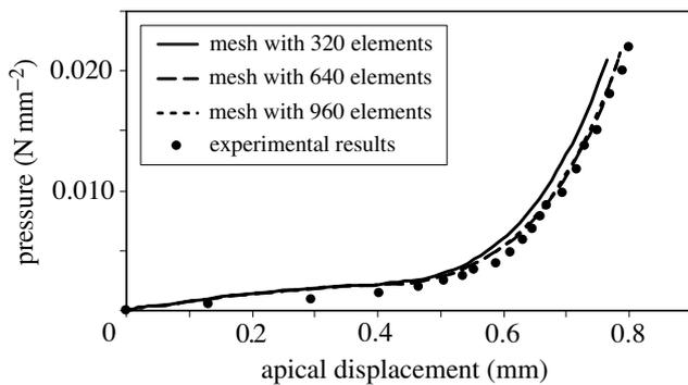
Figure 11. Effect of using finite-element meshes with different element densities.
