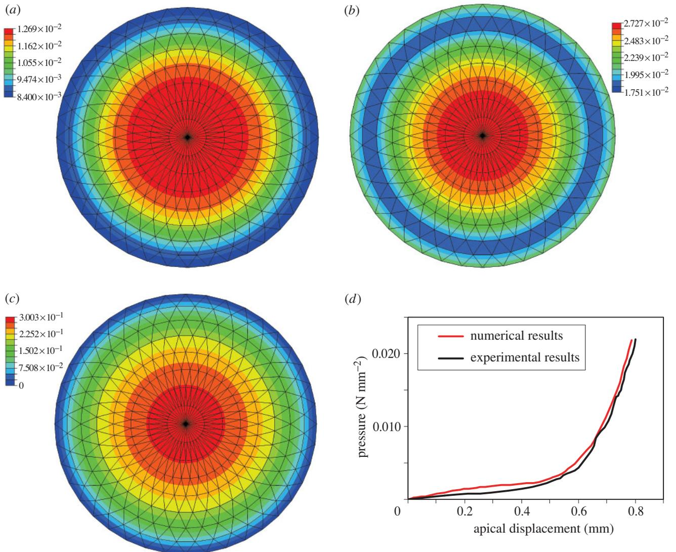
Figure 17. Example results of the numerical model under an IOP of 2 kPa (15.04 mmHg): (a) distribution of Mises strain ( $\text{N mm}^{-2}$ ); (b) distribution of maximum principal strain ( $\text{N mm}^{-2}$ ); (c) distribution of displacement (mm); (d) comparison between numerical and experimental IOP rise results.
