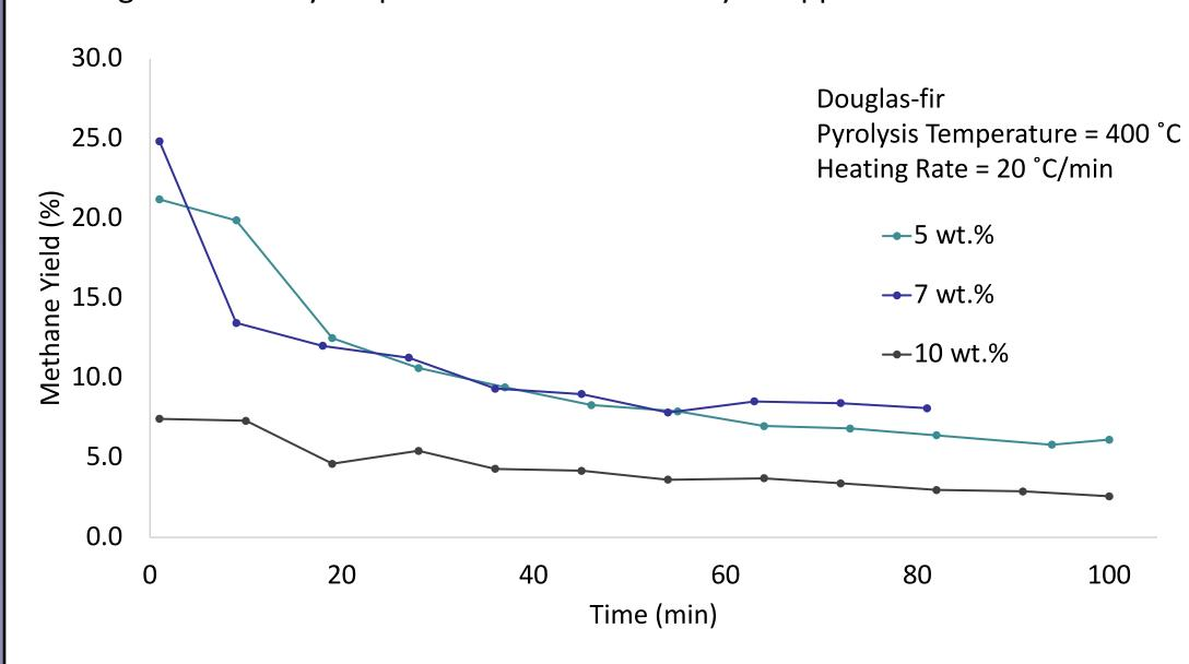
Methane yield is unchanged when nickel loading is increased from 5 wt.% to 7 wt.%, but decreases when it is further increased to 10 wt.%.
