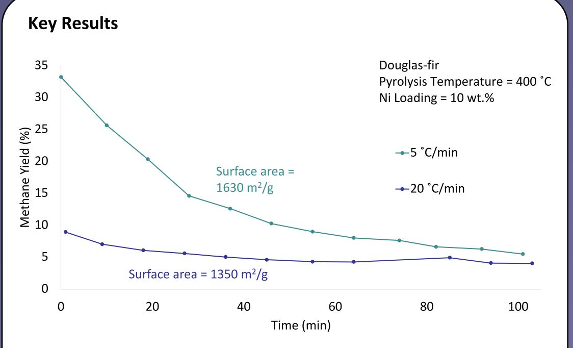
Methane yield increases as the heating rate during pyrolysis decreases.
