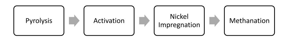
Research is required to determine the impact of biochar-based catalyst synthesis processes on their ability to catalyze the methanation reaction.
