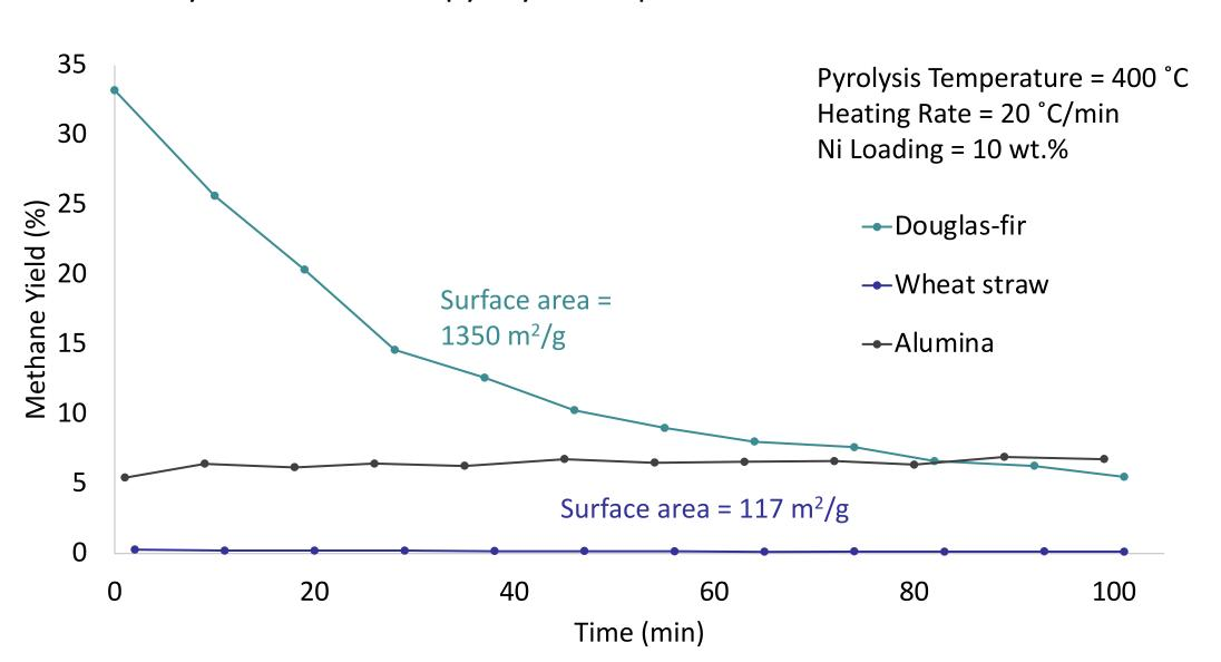
Methane yield is higher with Douglas-fir biochar vs. wheat straw biochar. Douglas fir initially outperforms standard catalyst support alumina.
