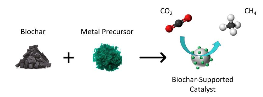
Biochar can be used as a catalyst support for the methanation reaction.
