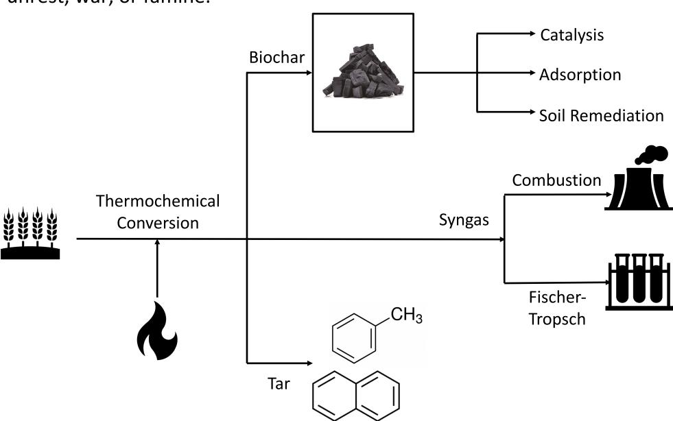
Biomass can be converted to green energy through thermochemical conversions creating biochar, tar or bio-oil, and syngas. Biochar is highly porous and tunable, making it desirable for several applications.
