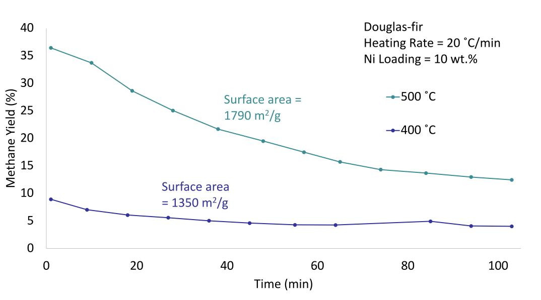
Methane yield increases as pyrolysis temperature increases.
