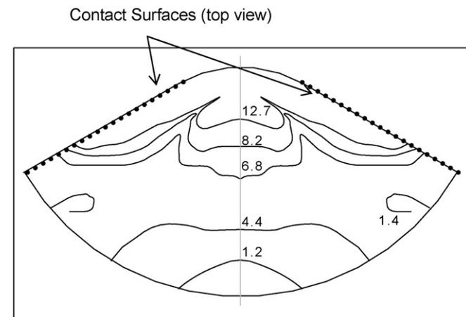
Fig. 7. The bending moment per unit length (mN)—in the vicinity of the contact area bending moment is maximum.
