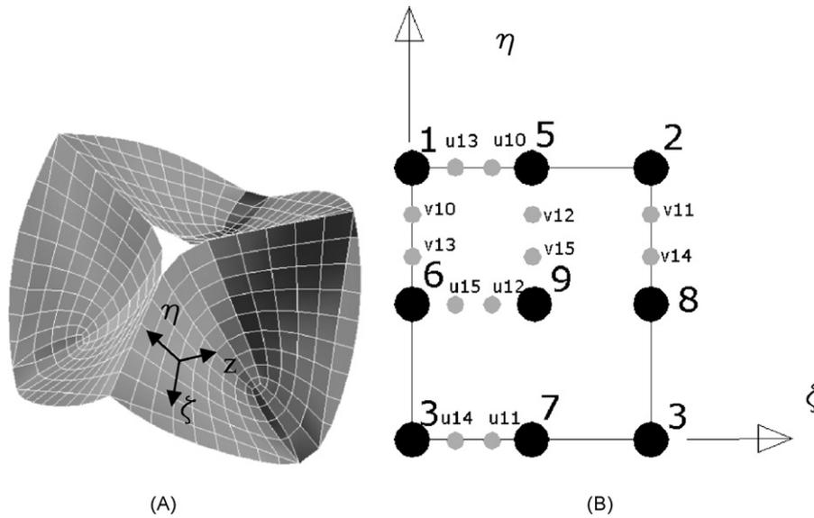
**Fig. 3.** The geometry of the HV leaflet tissue covered with only 183 high-order elements (A) and one single high-order element with demonstration of major and minor nodes (B).
