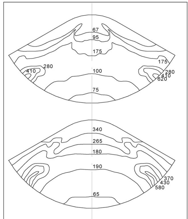
Fig. 5. The maximum principal stresses distribution over the leaflet tissue on the top layer (A) and on the bottom layer (B), with no contact considered between the two adjacent leaflets—values are in kPa.
