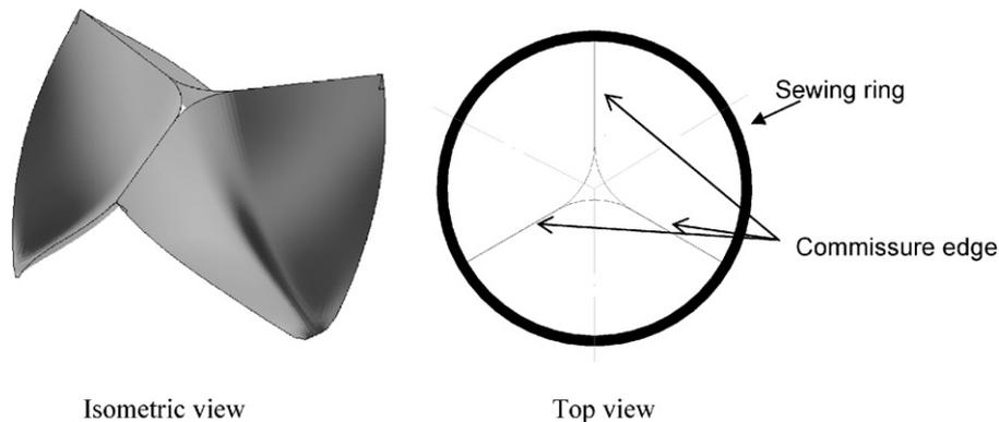
**Fig. 1.** The geometry of the HV leaflet tissue developed using Bezier type surfaces as described in [18].
