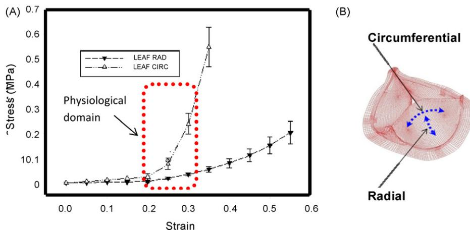
**Fig. 2.** The stress–strain curve for the porcine aortic HV leaflet tissue (A) in two principal directions as shown in (B). The radial direction in the figure corresponds to the longitudinal direction. It should be noted that the physiological range falls within the a strain between 20% and 30% [18].
