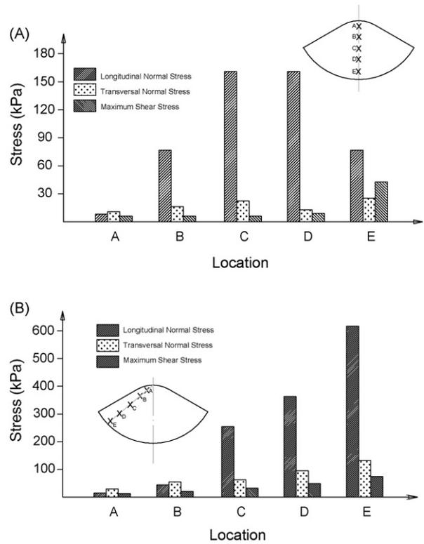
Fig. 8. Longitudinal normal stress, transversal normal stress and the maximum shear stress with respect to labeled locations, (A) on the midline of the leaflet, (B) on the line passing over the maximum values.
