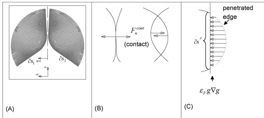
**Fig. 4.** (A) Geometry of the leaflets to be solved for a pushback contact solution, (B) surfaces before and after contact and (C) penalty method to contact force.
