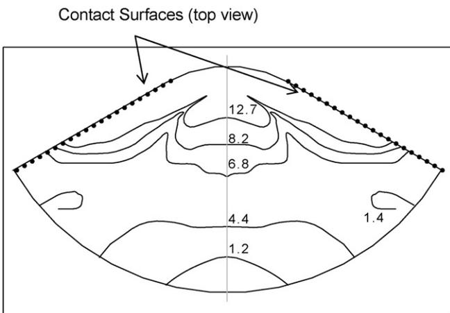
Fig. 7. The bending moment per unit length (mN)—in the vicinity of the contact area bending moment is maximum.
