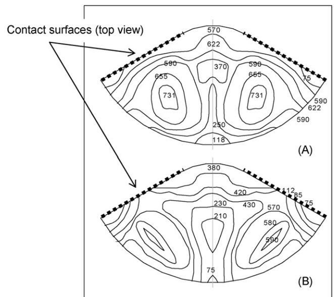
Fig. 6. The maximum principal stresses distribution over the leaflet tissue on the top layer (A) and on the bottom layer (B), accounting for the contact between the two adjacent leaflets—values are in kPa.
