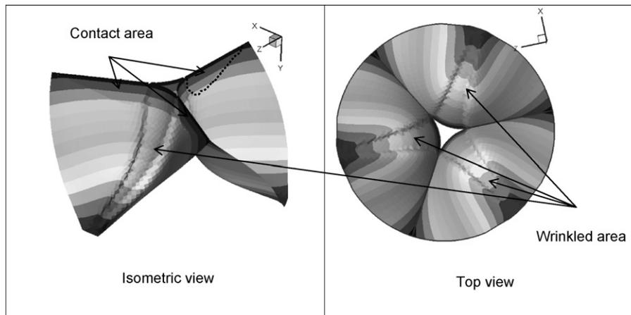
Fig. 9. Deformation of the HV leaflet in the closing phase. The contact area and the wrinkled area after deformation due to contact are shown with arrows.
