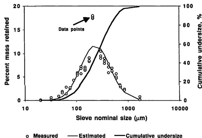
Fig. 2. Log-normal and cumulative undersize distributions of alfalfa grind particles used in this study.
