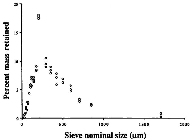
Fig. 1. The mass percentage of alfalfa grind retained on individual test sieves in relation to sieve openings.
