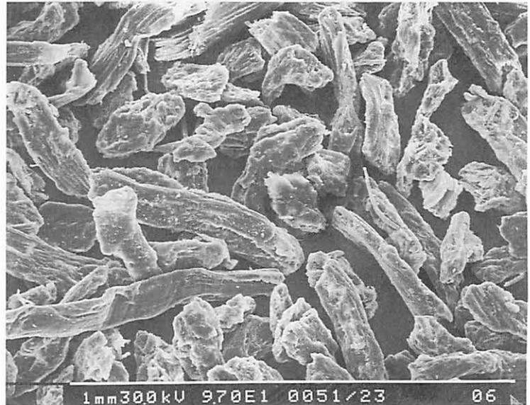
**Fig. 3. A SEM micrograph showing the alfalfa particles retained on the sieve of 90-µm opening.**
