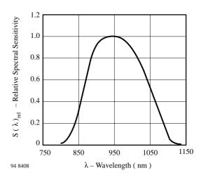
Figure 11. Relative Spectral Sensitivity vs. Wavelength
