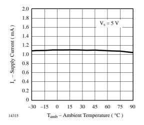
Figure 8. Supply Current vs. Ambient Temperature
