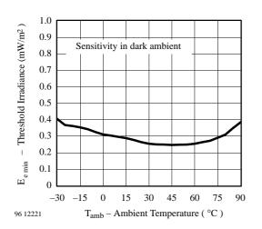
Figure 9. Sensitivity vs. Ambient Temperature
