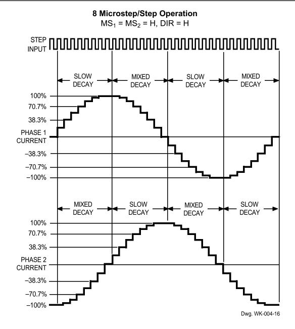
The mixed-decay mode is controlled by the percent fast decay voltage ( $V_{PFD}$ ). If the voltage at the PFD input is greater than  $0.6V_{DD}$  then slow-decay mode is selected. If the voltage on the PFD input is less than  $0.21V_{DD}$  then fast-decay mode is selected. Mixed decay is between these two levels.
