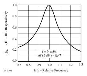
Figure 1. Frequency Dependence of Responsivity
