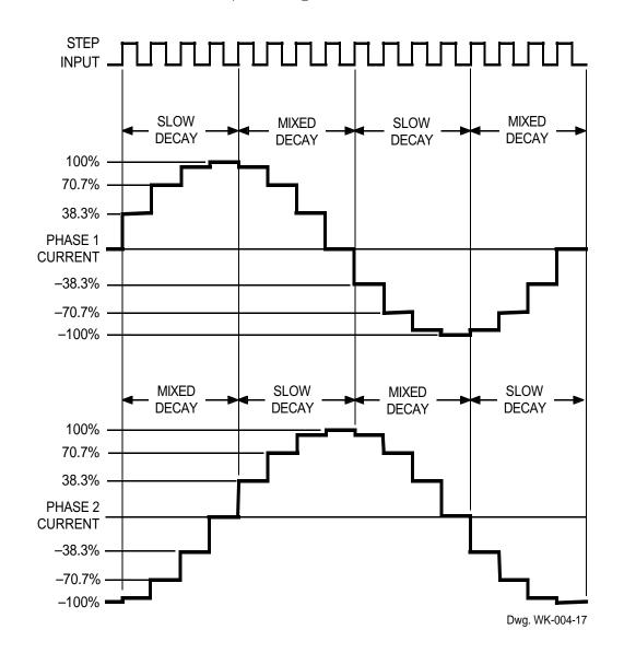
The mixed-decay mode is controlled by the percent fast decay voltage ( $V_{PFD}$ ). If the voltage at the PFD input is greater than  $0.6V_{DD}$  then slow-decay mode is selected. If the voltage on the PFD input is less than  $0.21V_{DD}$  then fast-decay mode is selected. Mixed decay is between these two levels.
