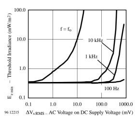
Figure 4. Sensitivity vs. Supply Voltage Disturbances
