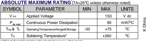
\*.200 inch (5 mm) from bottom of header for 3 secs max with heat sink
