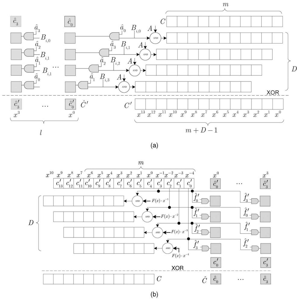
Fig. 12. Concurrent error detection for  $m = 11, D = k = l = 4$ : (a) the  $\times$  module, (b) the  $x^{-D}$  module.
