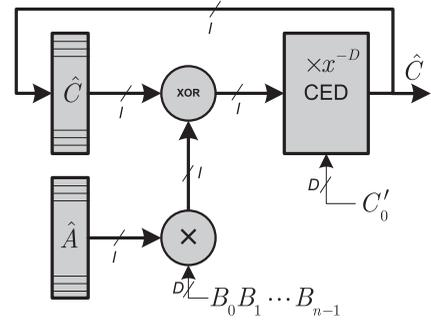
Fig. 5. Concurrent error detection in digit-serial Montgomery multiplication.
