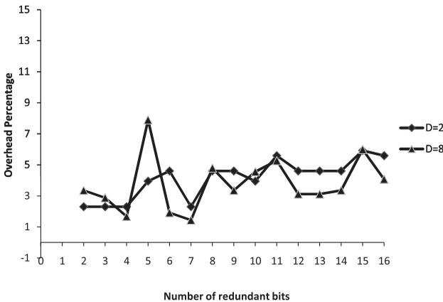
Fig. 8. ASIC implementation results for the time overhead in digit-serial Montgomery multiplication.
