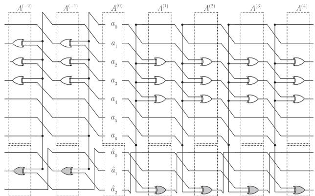
Fig. 13. Obtaining the matrix  $M$  with concurrent error detection for  $F(z) = z^7 + z^4 + z^3 + z^2 + 1$  using  $u = 2$ .
