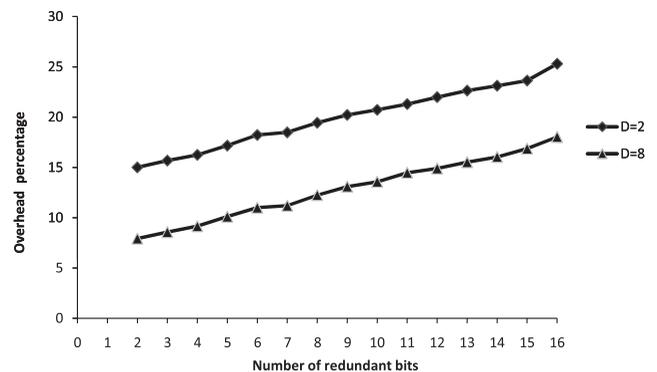
Fig. 9. ASIC implementation results for the area overhead in digit-serial Montgomery multiplication.
