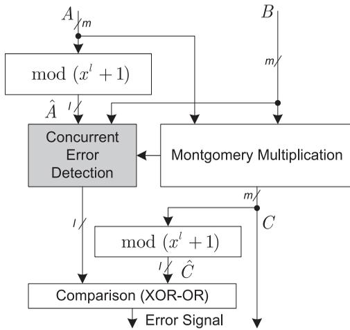
Fig. 1. Concurrent error detection scheme.
