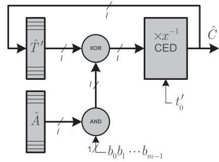
Fig. 4. Concurrent error detection for the bit-serial Montgomery multiplier.
