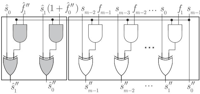
Fig. 6. Error detection in the  $x$ -module using  $l = 2$ .
