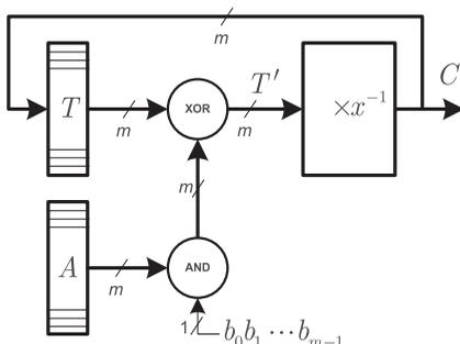
Fig. 2. Modified bit-serial Montgomery multiplication over  $GF(2^m)$ .
