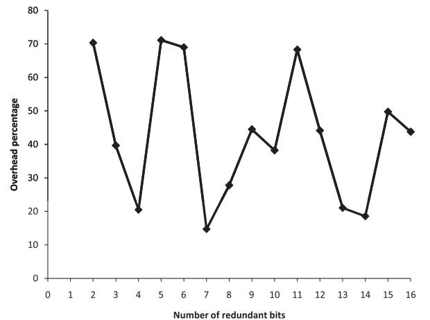
Fig. 11. ASIC implementation time overhead percentage of the concurrent error detection in bit-parallel Montgomery multiplication using  $F(z) = z^{163} + z^{72} + z^{71} + z^{70} + 1$ .
