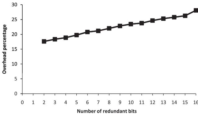
Fig. 7. ASIC implementation results for the area overhead in bit-serial Montgomery multiplication.
