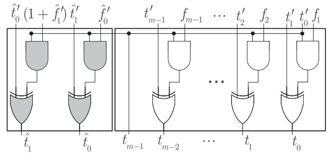
Fig. 3. The  $x^{-1}$ -module with error detection using  $l = 2$ . The gray gates show the overhead.
