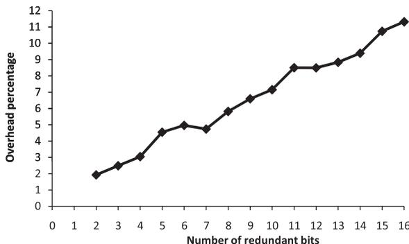
Fig. 10. ASIC implementation area overhead percentage of the concurrent error detection in bit-parallel Montgomery multiplication using  $F(z) = z^{163} + z^{72} + z^{71} + z^{70} + 1$ .
