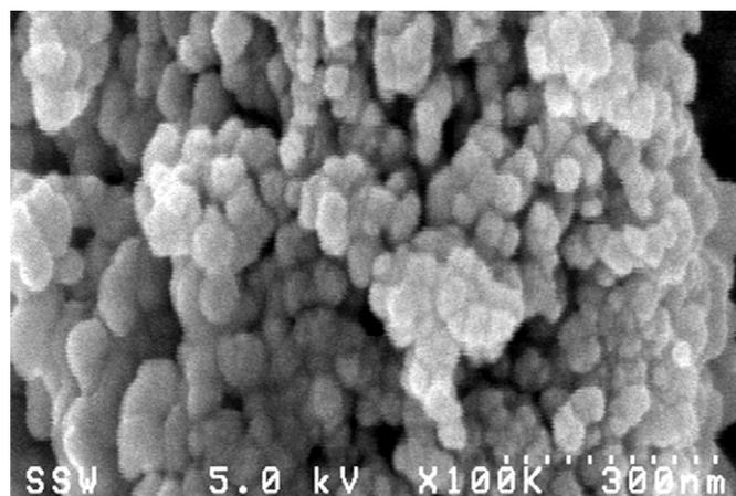
Fig. 1. Scanning electron photomicrograph of magnetite–maghemite nanoparticles (20–40 nm) at 100,000× magnification showing highly uniform sample.
