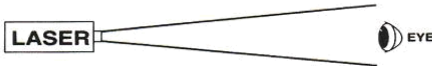
Figure 4 - Intrabeam viewing of direct (primary) beam. This type of viewing is most hazardous.
