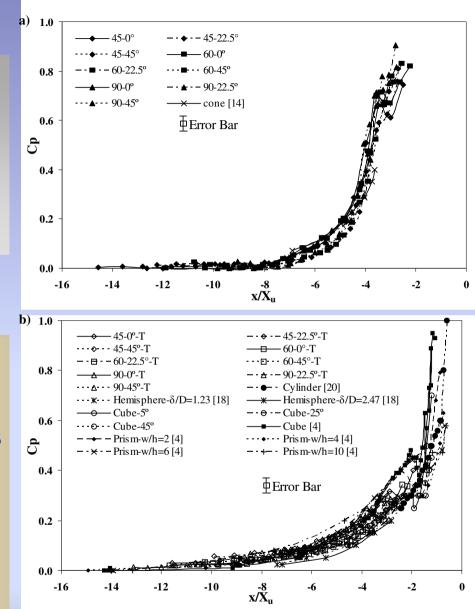
Upstream Cp distribution along z/h=0 with position scaled using  $X_u$  for bluff bodies in a) thin boundary layer, b) thick boundary layer
