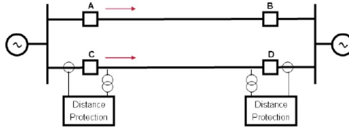
Figure 1: Example of Parallel Line System
