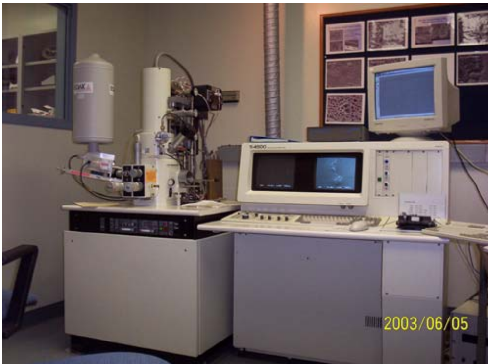
Figure 3.6.2.3 Picture of Hitachi S-4500 Field Emission SEM
