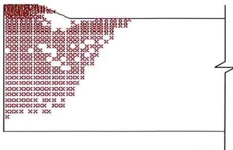
Figure 31. Plastic Zones and Velocity Fields at embankment heights of H=8.3 m and H=9.4 m
