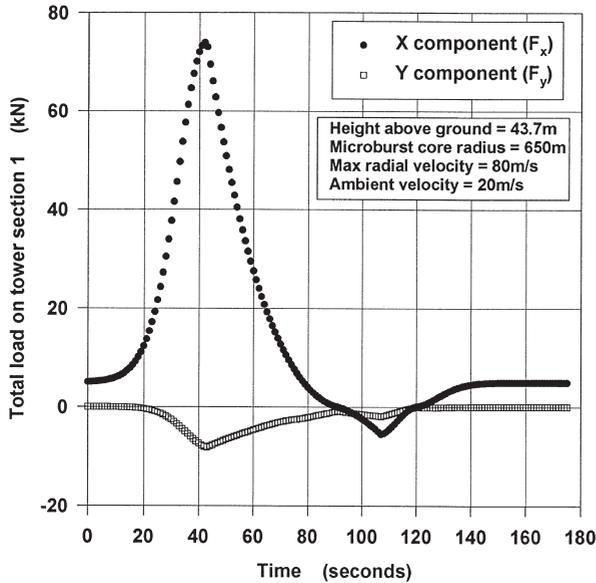
Fig. 11. Time history of the microburst horizontal wind loading components acting on Section 1 of the tower.
