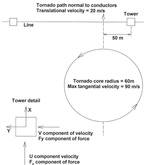
Fig. 6. Schematic of the modelled tornado characteristics and path relative to the tower.
