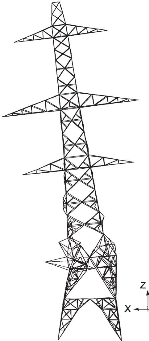
Fig. 14. Failure shape of the tower under the modelled tornado loading.
