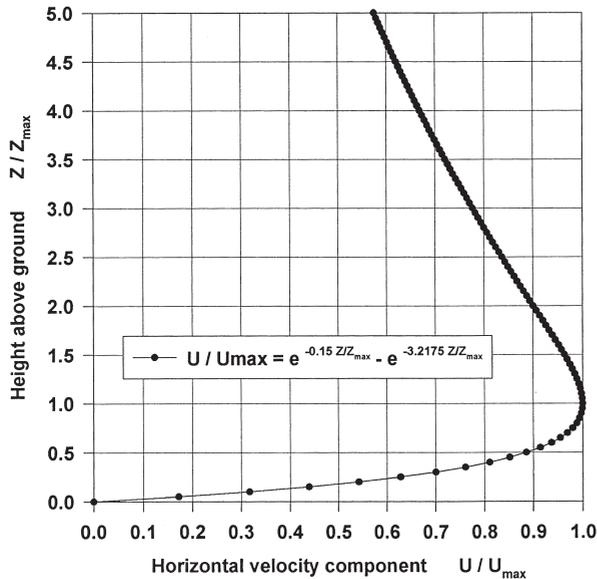
Fig. 3. Vertical profile of the horizontal radial outflow wind speed associated with a microburst.
