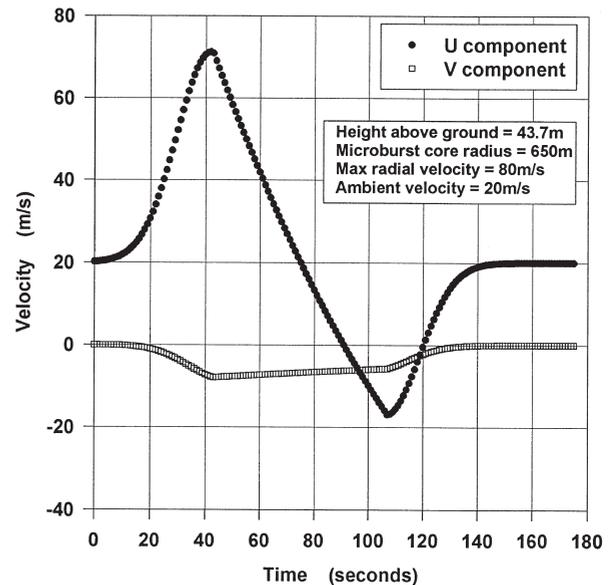
Fig. 10. Time history of the microburst horizontal wind speed components at the centre of Section 1 of the tower.
