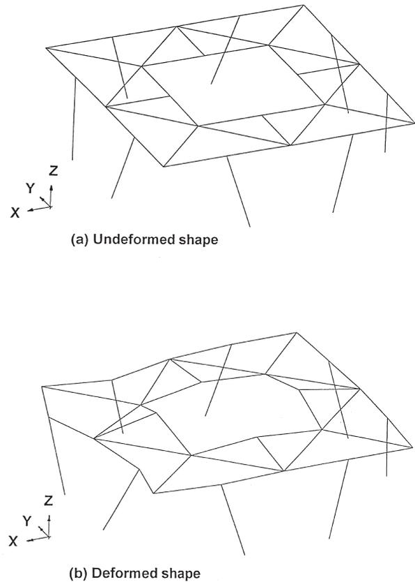
Fig. 15. Detail of the failure at the plan bracing between Sections 4 and 5.
