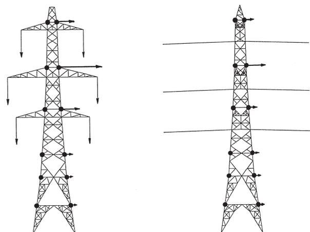
Fig. 5. Application of the wind loading to the tower.
