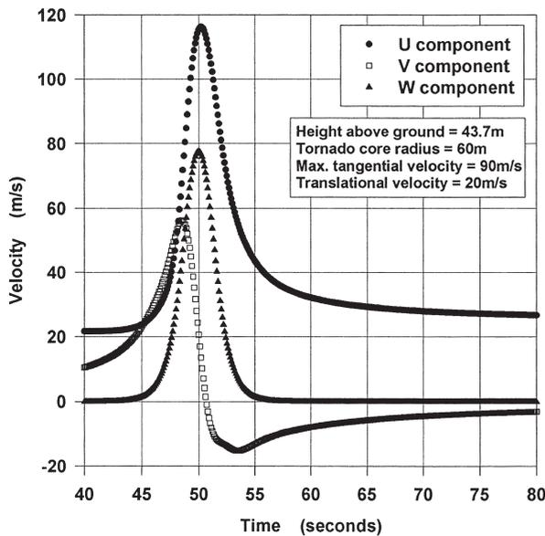
Fig. 8. Time history of the tornado wind speed components at centre of Section 1 of the tower.
