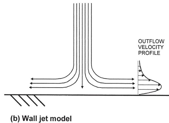
Fig. 2. Ring vortex and impinging wall jet models for a microburst.
