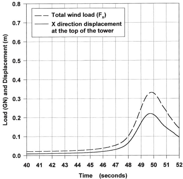
Fig. 16. Displacement of top of tower in the  $x$ -direction due to 50% of the tornado load.
