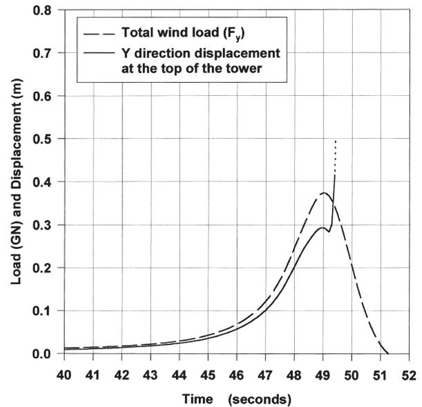
Fig. 13. Displacement of the top of the tower in the  $y$ -direction due to the tornado loading.
