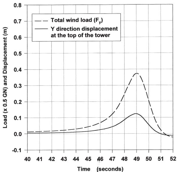
Fig. 17. Displacement of top of tower in the  $y$ -direction due to 50% of the tornado load.
