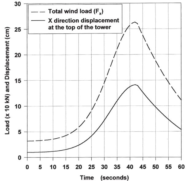
Fig. 18. Displacement of top of tower in the  $x$ -direction due to the microburst loading.
