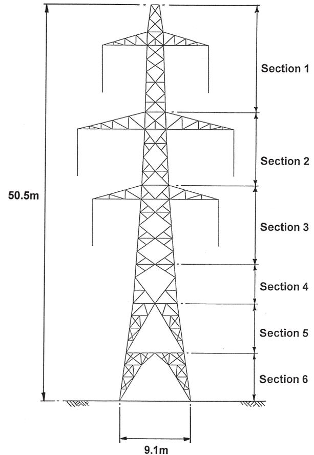
Fig. 4. Outline of the modelled lattice transmission tower.
