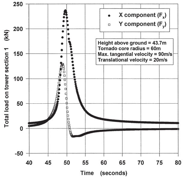
Fig. 9. Time history of the tornado horizontal wind loading components acting on Section 1 of the tower.
