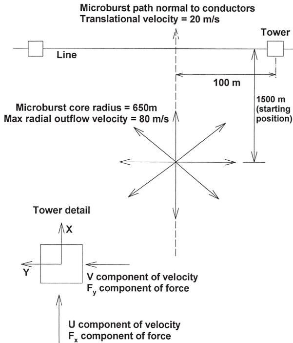
Fig. 7. Schematic of the modelled microburst characteristics and path relative to the tower.
