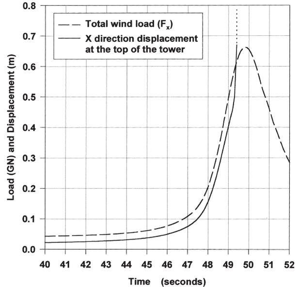
Fig. 12. Displacement of the top of the tower in the  $x$ -direction due to the tornado loading.
