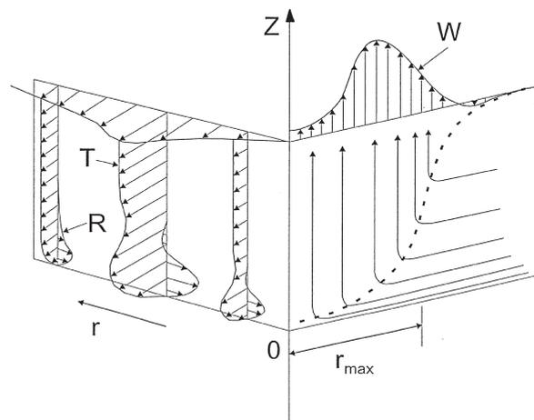
Fig. 1. Basic wind field structure of the modelled tornado [8,19] ( $R$ =radial velocity component,  $T$ =tangential velocity component,  $W$ =vertical velocity component).
