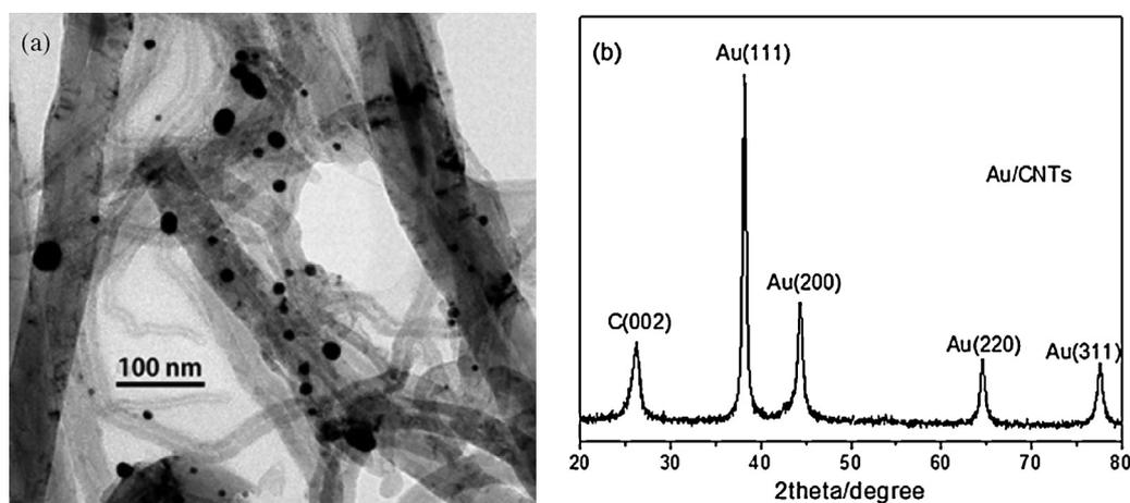
Fig. 1. (a) TEM and (b) XRD patterns of Au/CNTs.
