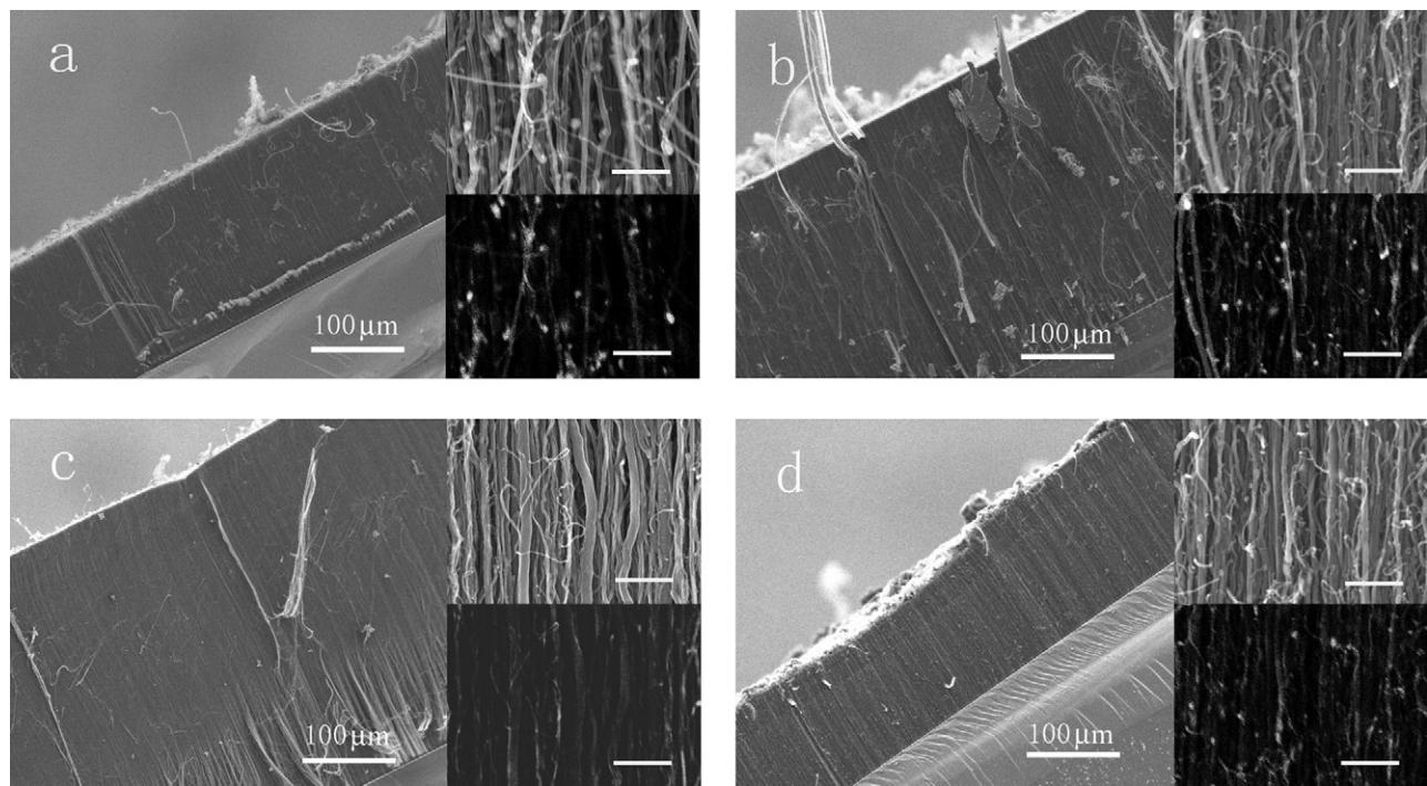
**Fig. 1.** SEM images of CNTs showing water effects (a) without water, (b) a little wet argon (10 sccm), (c) optimized amount of wet argon (150 sccm), and (d) excessive wet argon (700 sccm). All scale bars in inserted images are 500 nm. In each image, the bigger left image is low magnification SEM image, the up-right corner one is high magnification SEM image and the down-right corner one is back scattered electron image.
