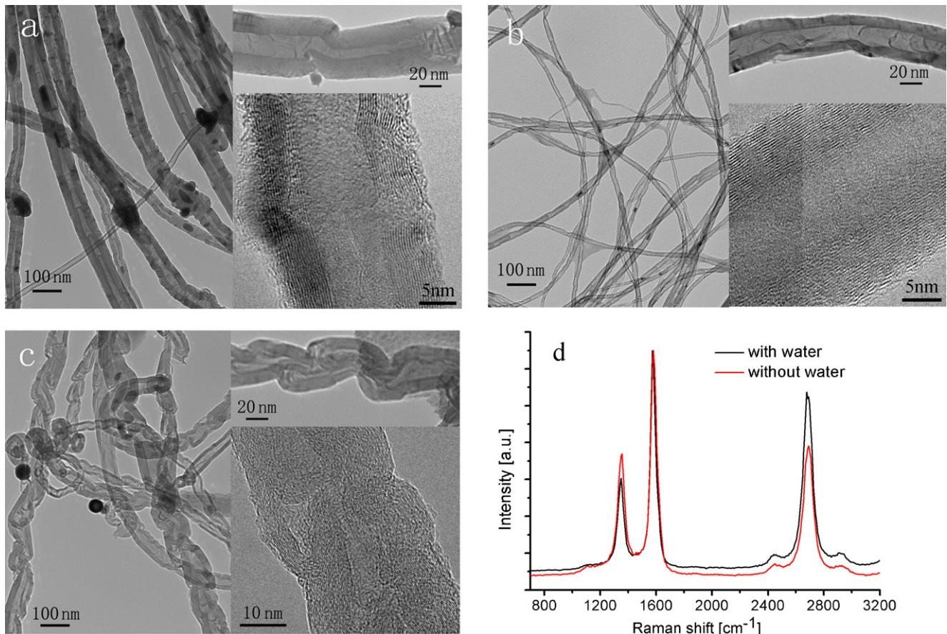
**Fig. 3.** TEM images and Raman spectra of CNTs using different wet argon flows. (a) Dry argon, (b) 150 sccm wet argon, (c) 700 sccm wet argon, and (d) Raman spectra of CNTs with dry argon and 150 sccm wet argon.
