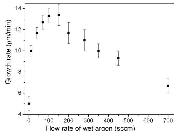
**Fig. 2.** Growth rate of MWCNTs as a function of flow rate of wet argon.
